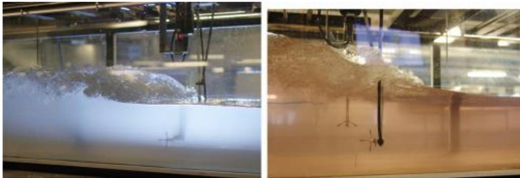
Figure 5. Demonstration of velocity measurement with the fixed ADV. Reprinted with permission from Leng and Chanson (2018). Copyright 2018, Elsevier.
