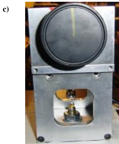
Figure 2.2: Pictures of a) the laboratory setup showing the circular aperture placed over the stimulus presentation monitor; mechanical knob for the subjects to make a two-alternate forced choice response; head rest and bite bar used to stabilize the subjects' head; b) experimental setup with a model subject, and c) mechanical knob for subjects to rotate in the clockwise or counterclockwise direction to make a two-alternate forced choice in order to indicate the direction of perceived orientation change of the probe in comparison to the previously presented target.
