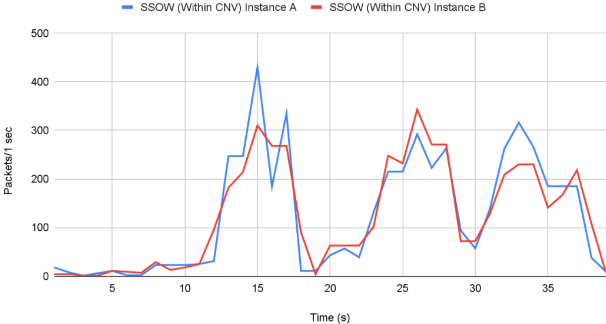
Figure 22: Two Representative Instances of Server-Side Originating DTW Watermarks as Observed at CNV
