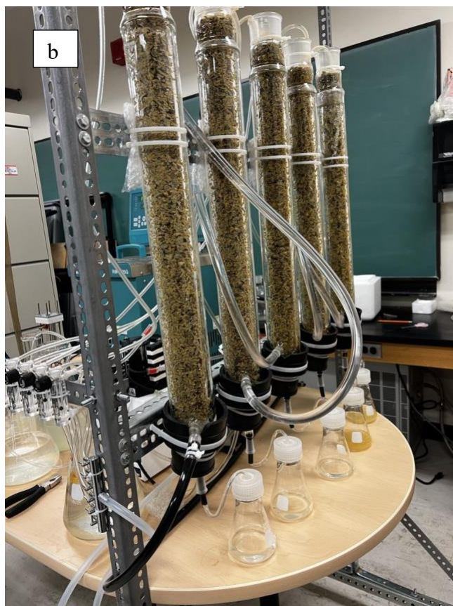
Figure 5.2. a) process flow diagram of column test biooxidation; b) experimental setup; c) temperature control system;and, d) aeration flowmeter and controlling valve for each column.
