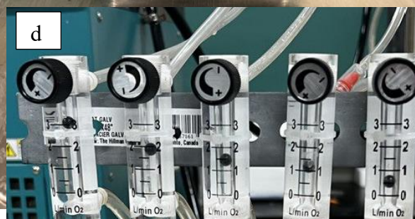
Figure 5.2. a) process flow diagram of column test biooxidation; b) experimental setup; c) temperature control system;and, d) aeration flowmeter and controlling valve for each column.
