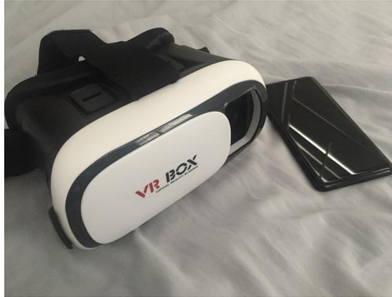
**Figure 4.4:** These were the Head mounted display, VR box, as well as the phone, Google Pixel 2, that were used to conduct the experiment. The pixel phone is inserted in the VR box and the screen was used to display an augmented image of the world to the wearer of the headset.
