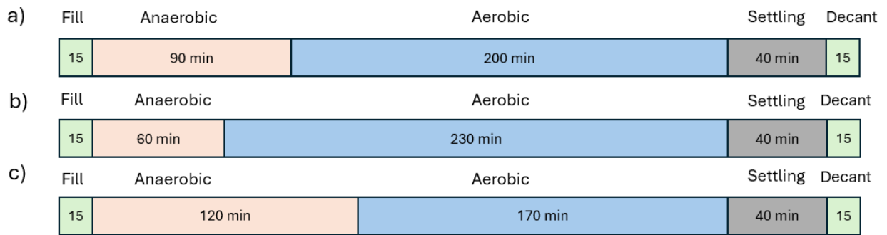
Figure 3-2: SBR cycle phase breakdown for different experimental scenarios to achieve the thesis objectives
