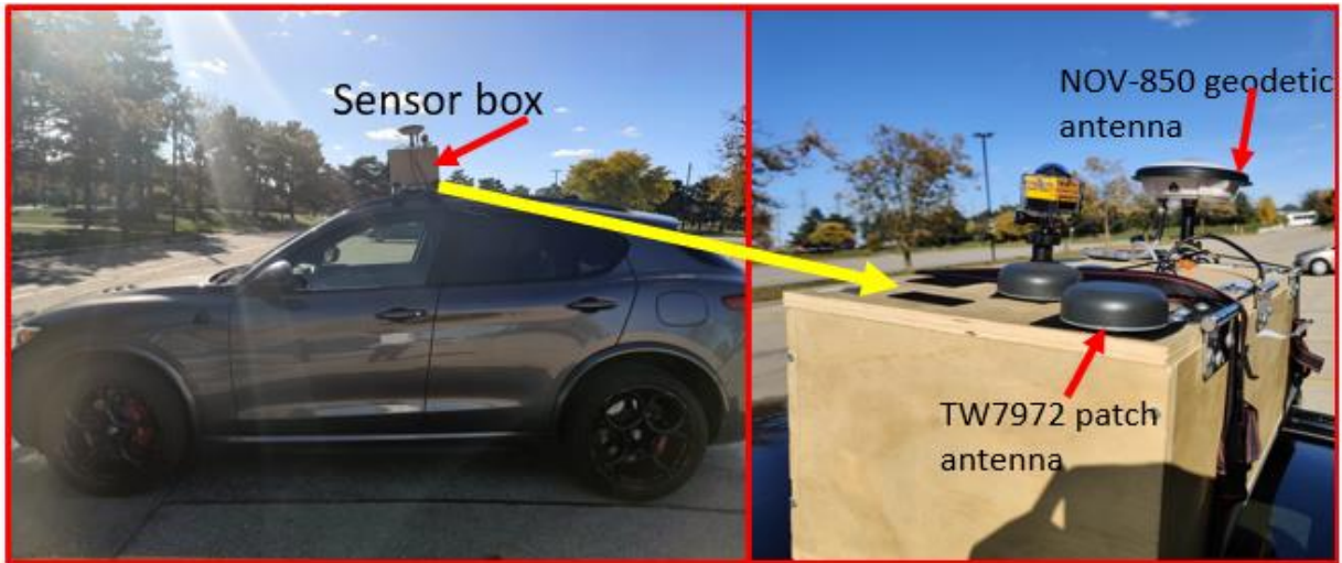
Figure 5-2: Rover experiment setup on car roof
