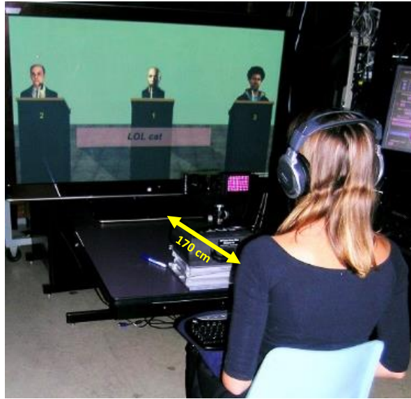
Figure 5.2: Experimental setup. The participant sat in-front of a TV screen, while her eyes were tracked by EyeLink 1000.
