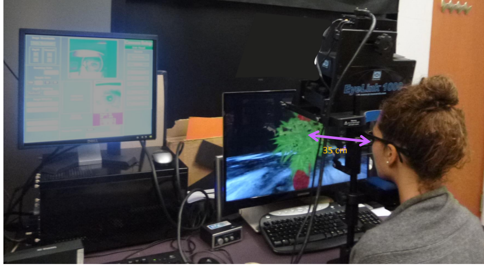
Figure 4.4: Experimental setup. The participant sat in front of the 3D display (partially visible beyond the tower mount) with her head fixed by the tower mount provided with the EyeLink 1000.
