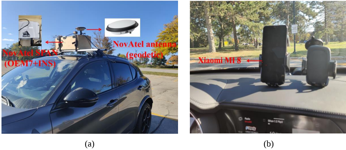
Figure 3.3 Photos of experimental setup. (a) experimental vehicle and setup, (b) experimental smartphones
