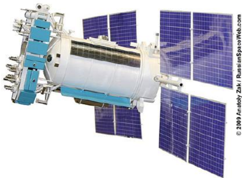
Figure 2.1 Russian GLONASS satellite ( www.russianspaceweb.com/uragan.html )
