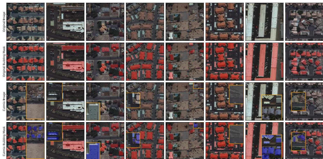
Figure D.1: CutMix examples. The first row shows the original image, followed by the original image overlaid by the ground truth building footprints in red. In the third row we can see the new images with the random CutMix patch and finally in the last row we present the final augmented images with the building annotations of the CutMix patch shown in purple.
