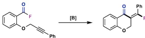
Figure 2.11. Initial substrate design for testing borane LA for atom-economical carbofluorination reactions.
