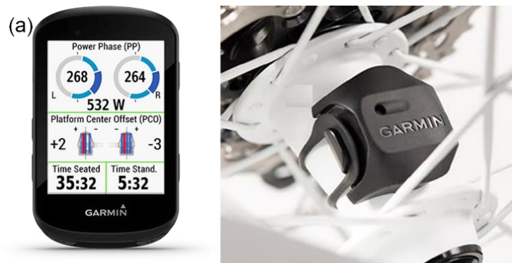
Figure 7: (a) Garmin Edge 530 and (b) Speed Sensor (Garmin, 2024)
