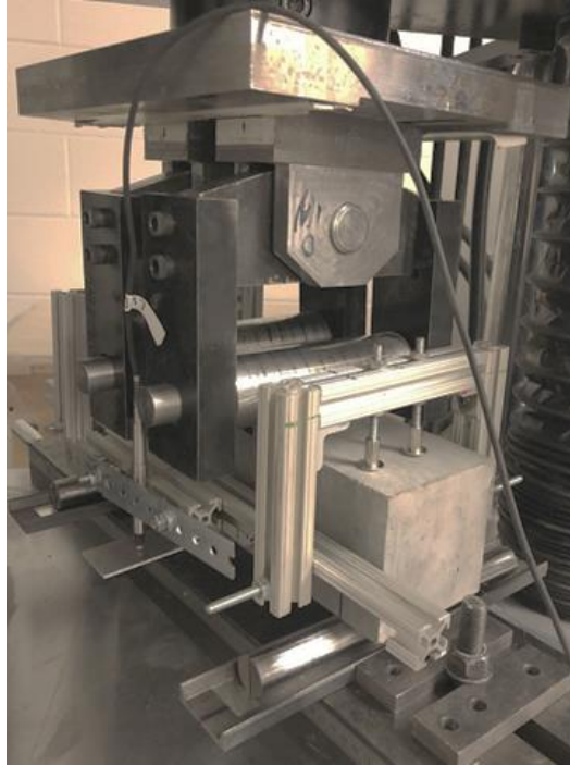
Figure A-106. Experimental test setup of four-point bending test
