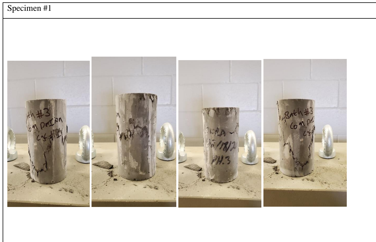
Figure A-119: Batch 3, Compression failure type summary
