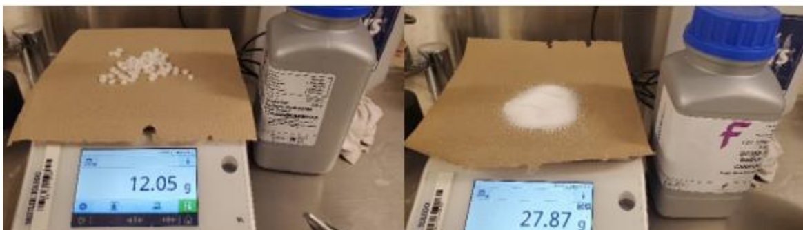
Figure 12: (a) Sodium Hydroxide used for RCPT (b) Sodium Chloride used for RCPT
