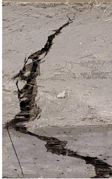
Figure 5: Bridging Behavior of Steel Fiber
