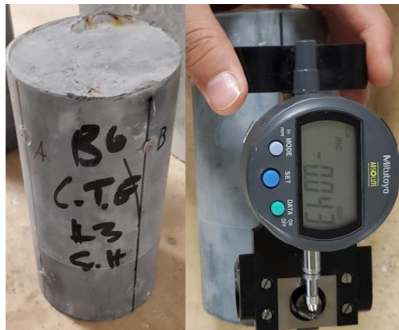
Figure 41: Demec gauge and gauge readings on C.T.E specimens.
