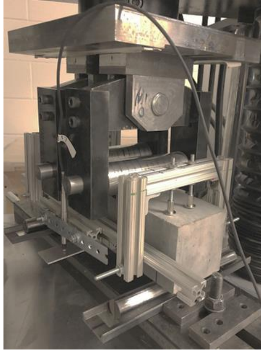
Figure A-109. Experimental test setup of four-point bending test
