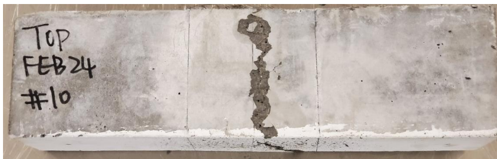
Figure 31: Marks used to align the prism perfectly perpendicular.
