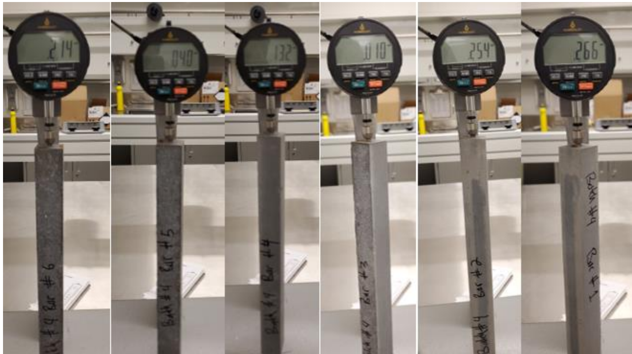
Figure 16: Sulfate bars in length comparator.
