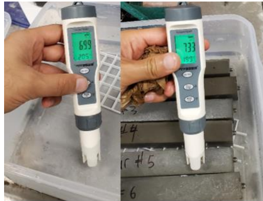
Figure 18: (a) PH reading of distilled water, (b) PH reading of sulfate solution with specimen's bars
