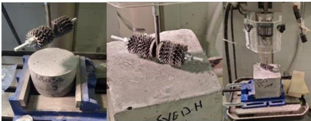
Figure 6: (from Left to right) (a) Abrasion Specimen 100mm × 150mm (Half Cut Specimen); (b) rotating stainless steel wheel; (c) Abrasion Cube Specimen 100mm × 100mm × 150mm)
