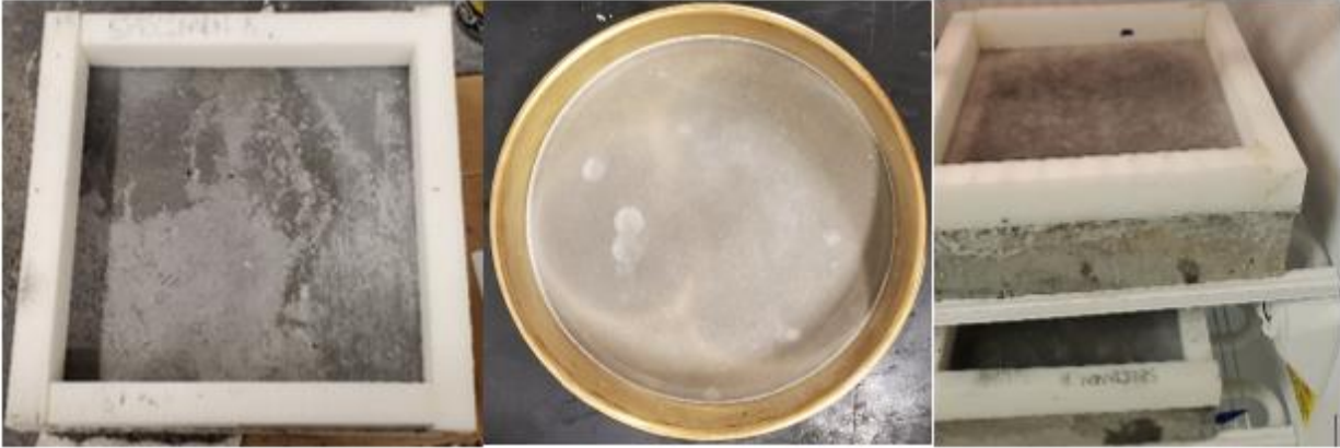
Figure 7 (from left-right): (a) Salt Scaling specimen dyke placement. (b) 80µm sieve used to filter the solution. (c) Salt scaling specimens in freezing condition.
