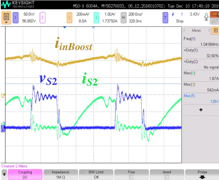
Fig. 4-9: Switch  $S_2$  waveforms and boost inductor current
