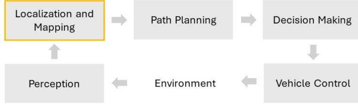
Figure 1.1 Key Modules in an Autonomous Vehicle System.
