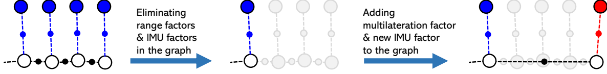
Figure 4.5 Description of the Add-After-Eliminating strategy for adding a multilateration factor to the factor graph.
