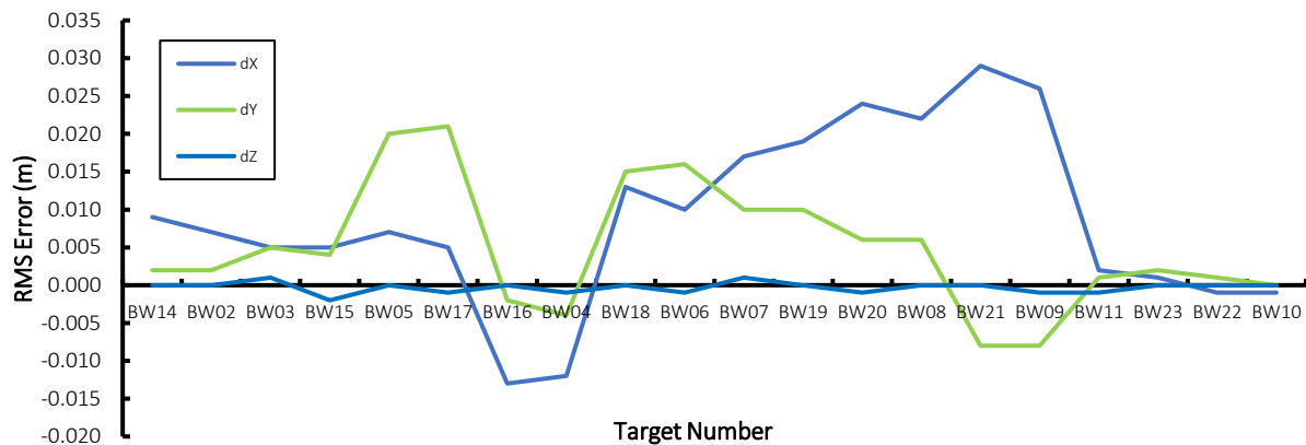
Figure 4.10: The RMS Error Produced By The TLS Technique compared to the land surveying method
