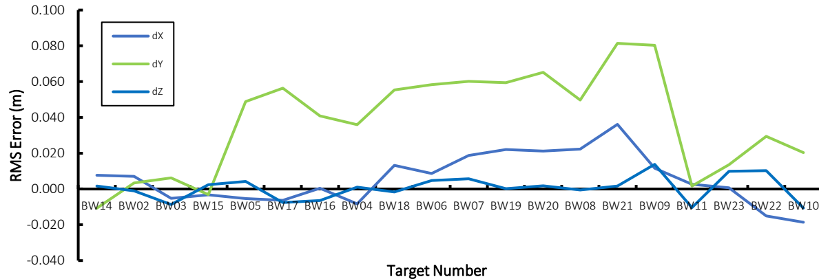
Figure 4.9: The RMS Error Produced by The CRP Technique compared to the land surveying method
