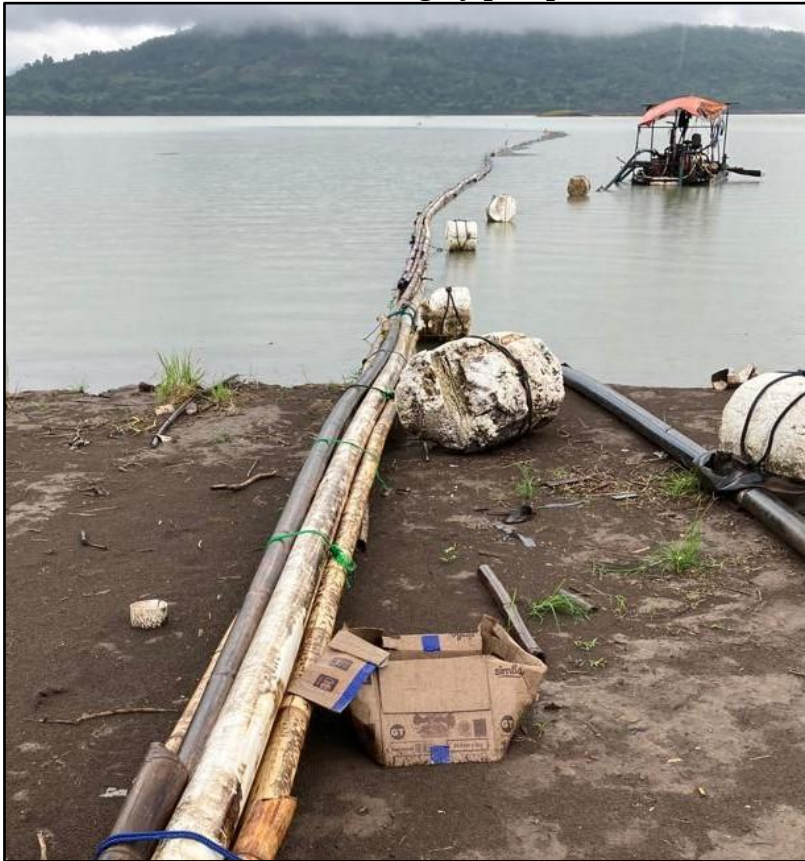
Photo 3.1. Current sand mining by pump in Bili-Bili reservoir (rainy season, 2022).
