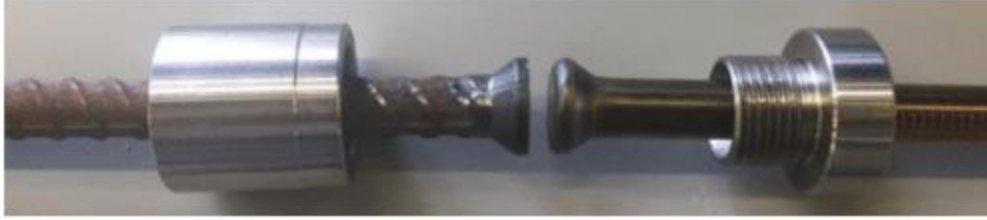
Figure 5.2 Headed #13 rebar (left) and SMA (right) with mechanical coupler (Morcos & Palermo, 2018).
