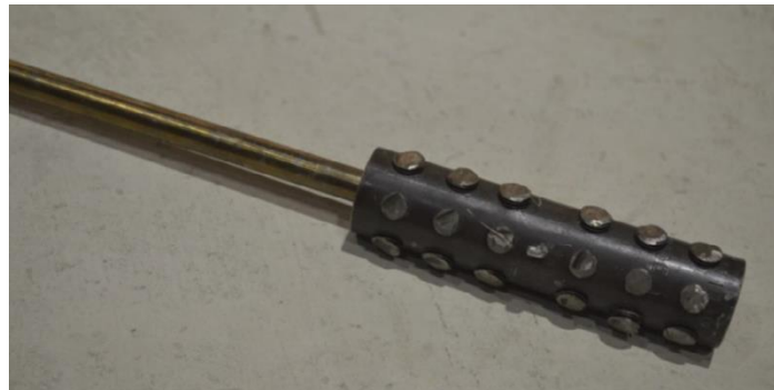
Figure 2.3: Mechanical screw coupler after modifications to solve premature failure and slipping (Abdulridha & Palermo, 2017).
