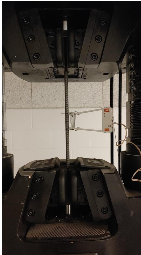
Figure 5.11 UTM setup with rebar and extensometer at beginning of tension test.
