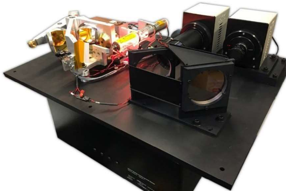
Figure 4-16: Optical bench setup of the IFTS instrument payload mounted on the vibration isolation platform.
