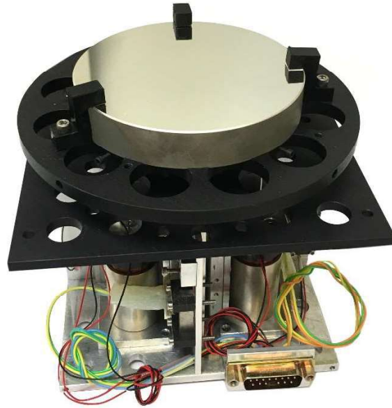
Figure 5-1: A linear two-axis tilt mirror image stabilizer pointing system.
