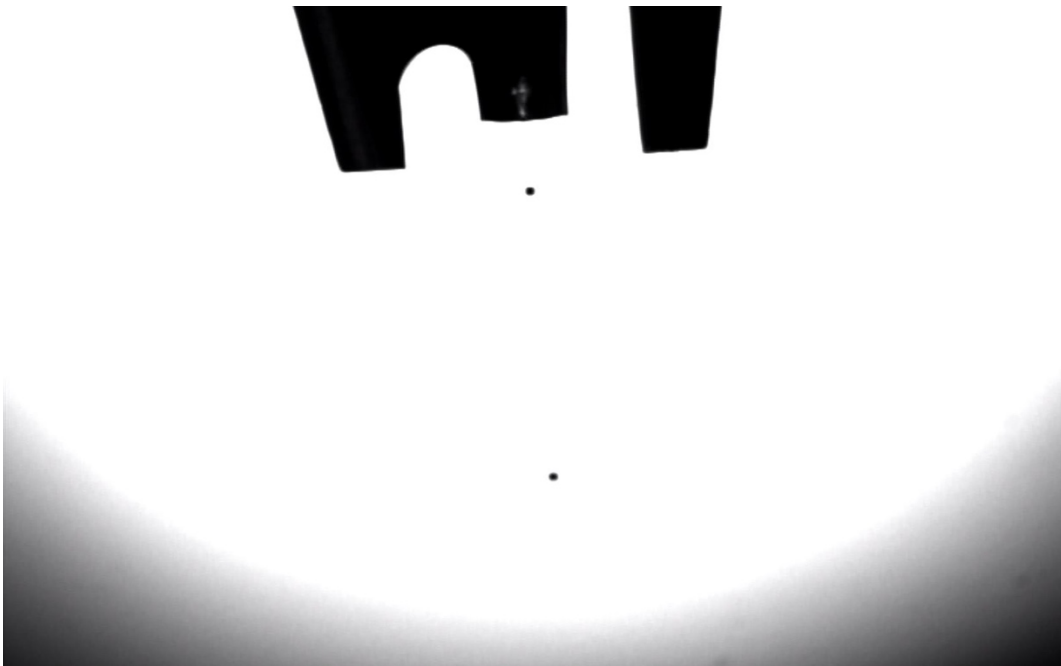
Figure 3-2. The satellite-free production of spherical droplets and a stream of ejected PEDOT:PSS ink.
