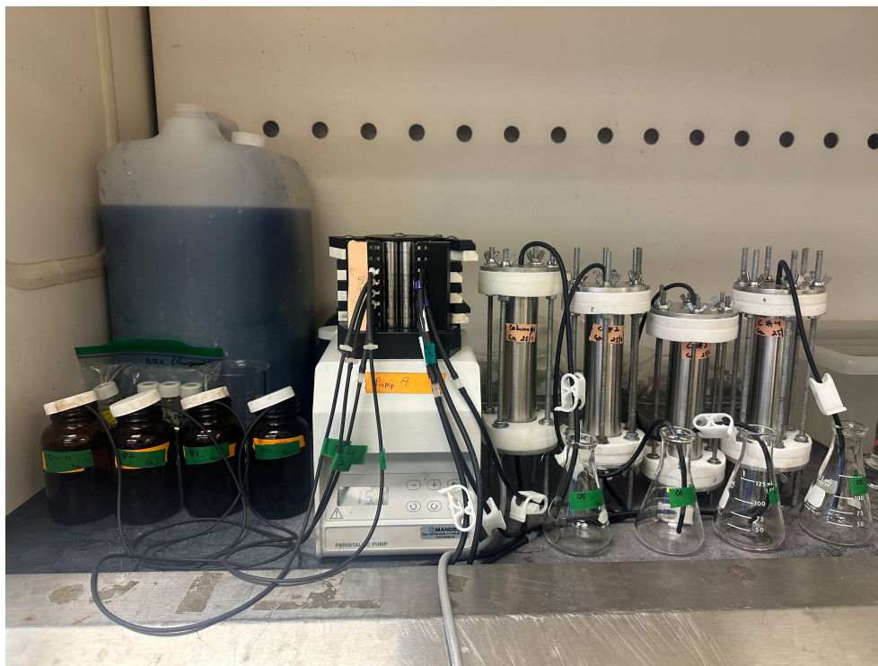
Figure F7: Stainless steel columns with PPE tubing.
