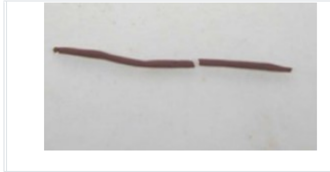
Figure A1: 3 mm rolled thread to measure plastic limit.
