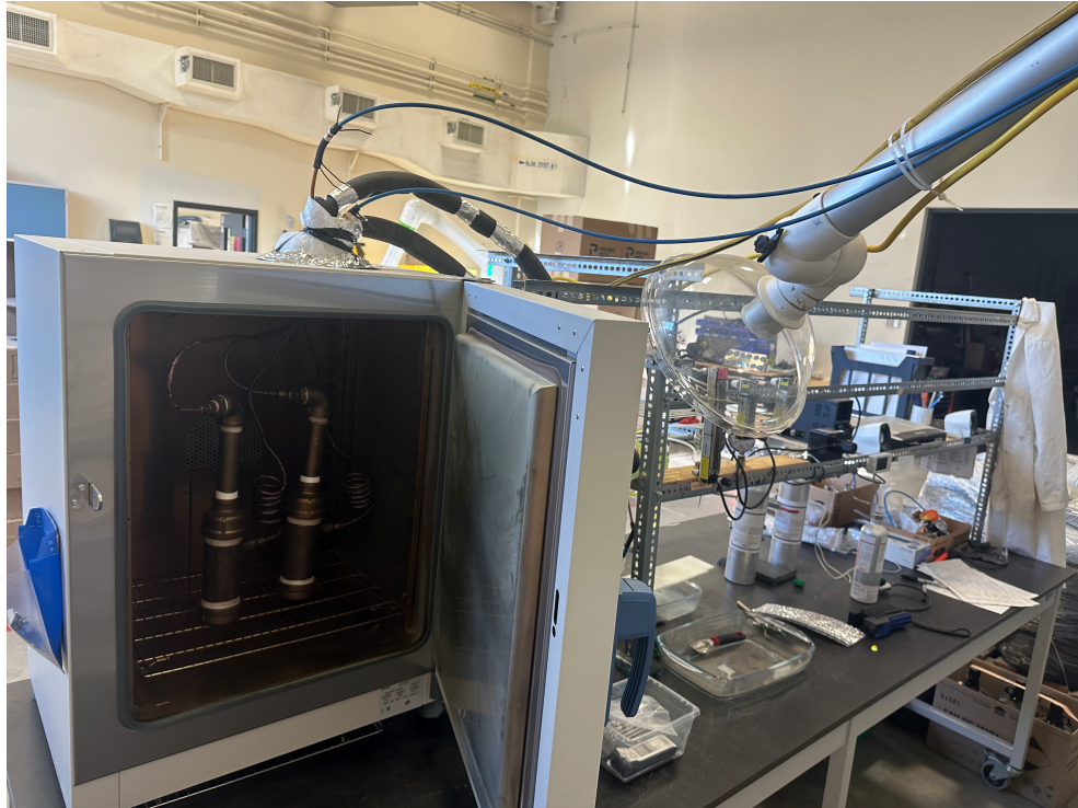
Figure F6: Stainless steel columns in an airtight chamber.
