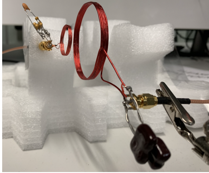
Figure 4.21: Implemented inductive link with wire-wounded coils for visual prosthesis application.
