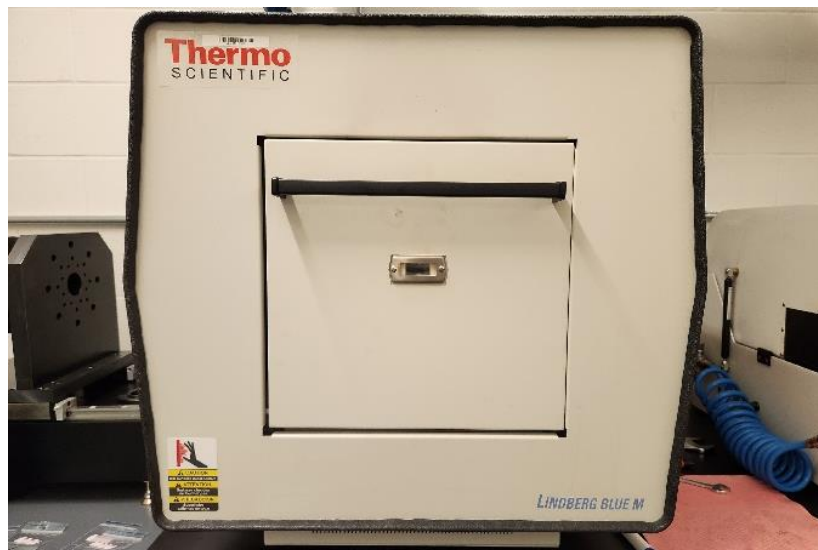
Figure C-1: Thermo Scientific Lindberg Blue M furnace used for static high temperature exposure testing
