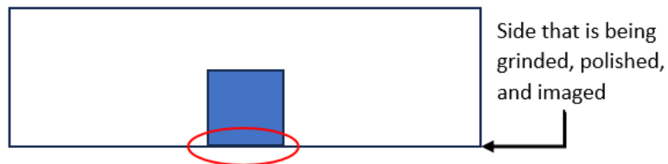
Figure 3-18: Images demonstrating which impacted surface was mounted for grinding, polishing, and imaging
