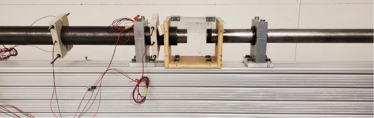
Figure 3-4: Direct Hopkinson Pressure Bar setup
