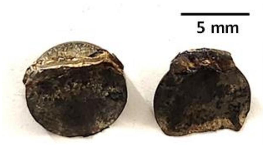
Figure 3-34: Images of sample T200-ZB: 200°C fracture with impact momentum 21.99 kg m/s showing failure and pigment change due to temperature exposure
