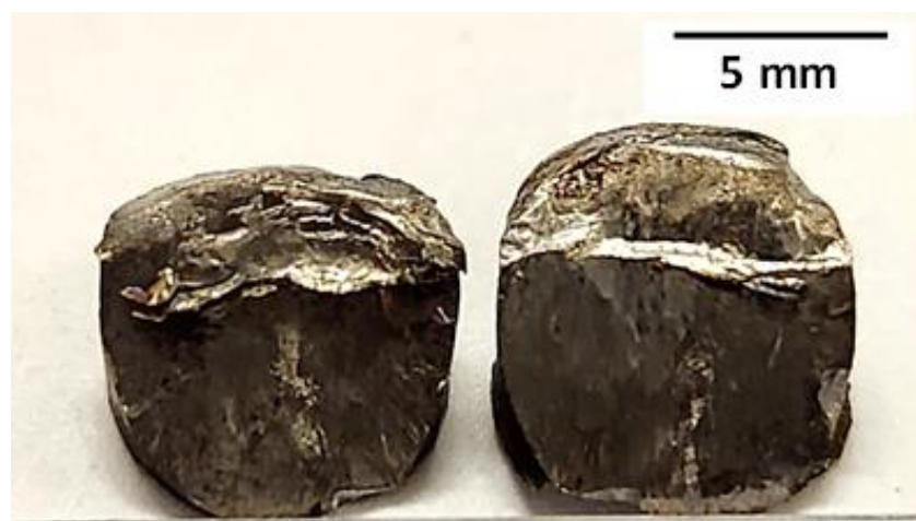
Figure 3-29: Image of sample RT10-A: Room temperature fracture with impact momentum 21.72 kg m/s showing failure
