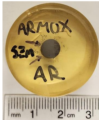
Figure 3-19: Images demonstrating the impacted mounted surface for grinding, polishing, and imaging
