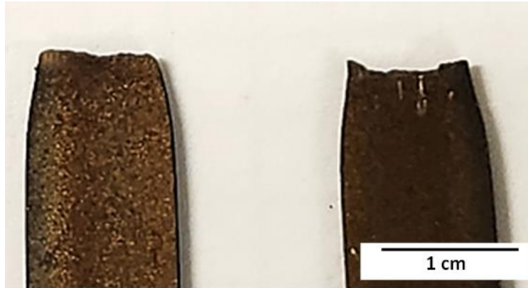
Figure 4-13: Quasistatic tensile test 300°C fracture sample Q300-A
