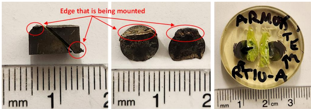
Figure 3-20: Images demonstrating which fractured corners were mounted for grinding, polishing, and imaging
