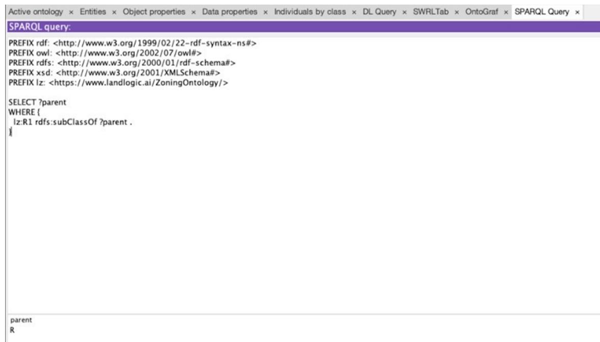
Figure 4.3 SPARQL query and result identifying the equivalent zoning class of R1.
