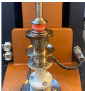
Figure 3.8 Testing the rheological properties of the post-crosslinked alginate.
