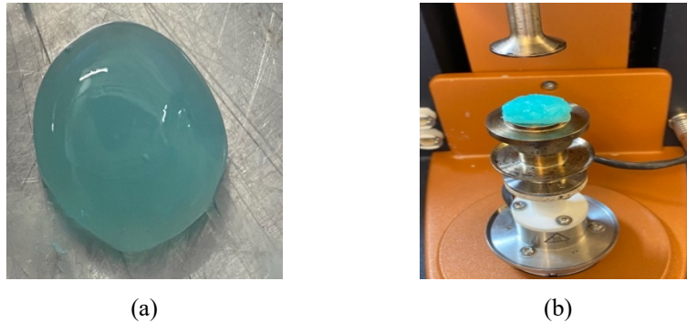
Figure 3.33 Crosslinked nanofibre tested for its rheological properties: (a) the coupon before tested, and (b) the coupon after a compression test.
