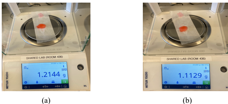
Figure 3.58 The printed coupon as it was : (a) removed from the gelatin slurry, and (b) an hour later.
