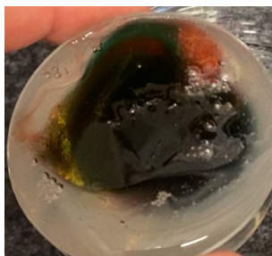
Figure 5.4 Finished printing product without the proper extrusion parameters set.
