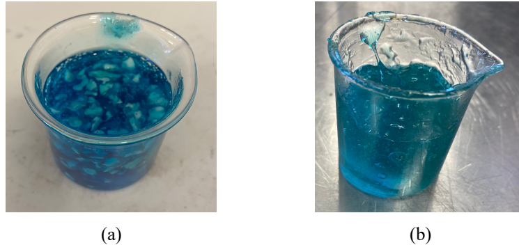
Figure 3.3 The creation of alginate biomaterial: (a) semi-mixed (b) fully incorporated.
