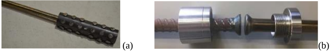
Figure 2.11 Mechanical couplers: (a) Original study by Abdulridha and Palermo (2013); and (b) study by Morcos and Palermo (2019).
