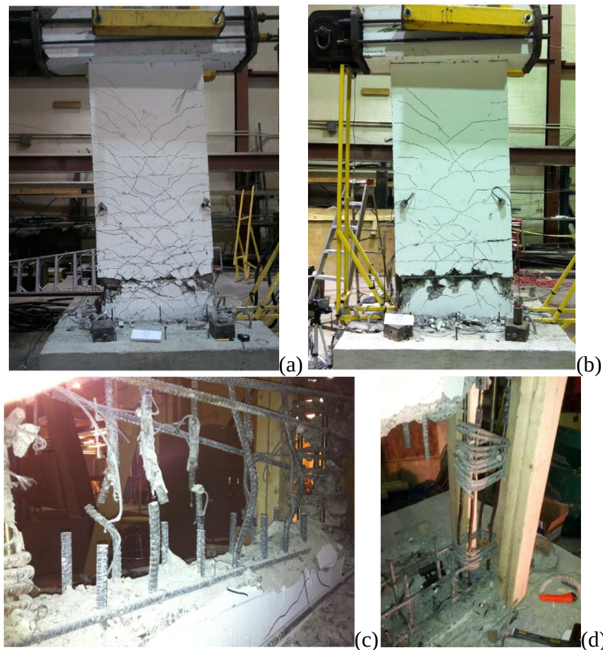
Figure 2.9 Conditions of the walls at failure: (a) W1-SR; (b) W2-NR (Abdulridha and Palermo, 2013); (c) rupture and buckling of steel reinforcement in the web of W2-NR; and (d) buckling of SMA bars in the boundary zone for W2-NR (Zaidi, Palermo and Dragmeriscu, 2016)
