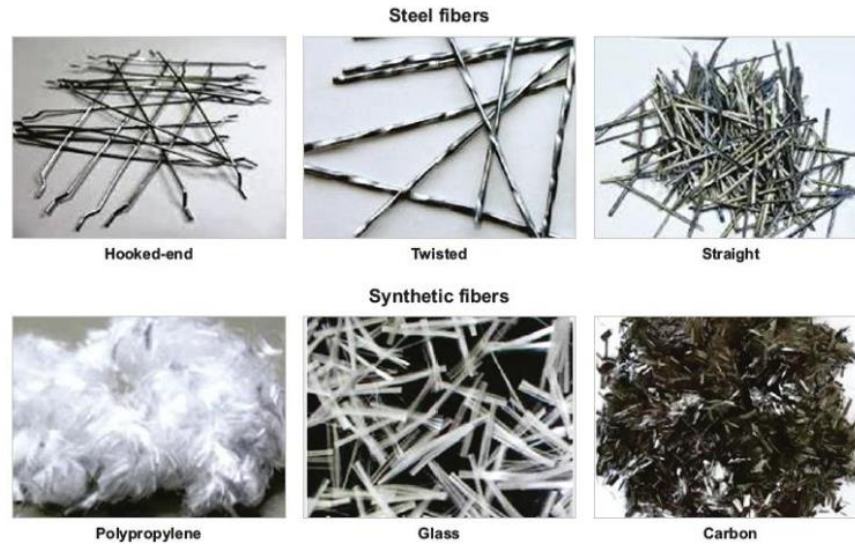
Figure 1.14 Different types of steel and synthetic fibers added to the concrete matrix (Buttignol, Sousa and Bittencourt, 2017)
