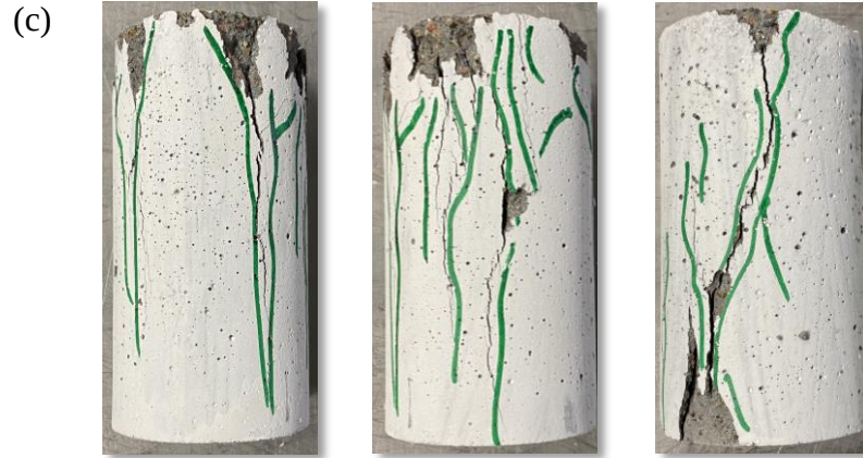
Figure 5.1 Compression cylinder failure mode: (a) ECC-RSWS-R; (b) ECC-RSWN; and (c) SCC-RSWS-R
