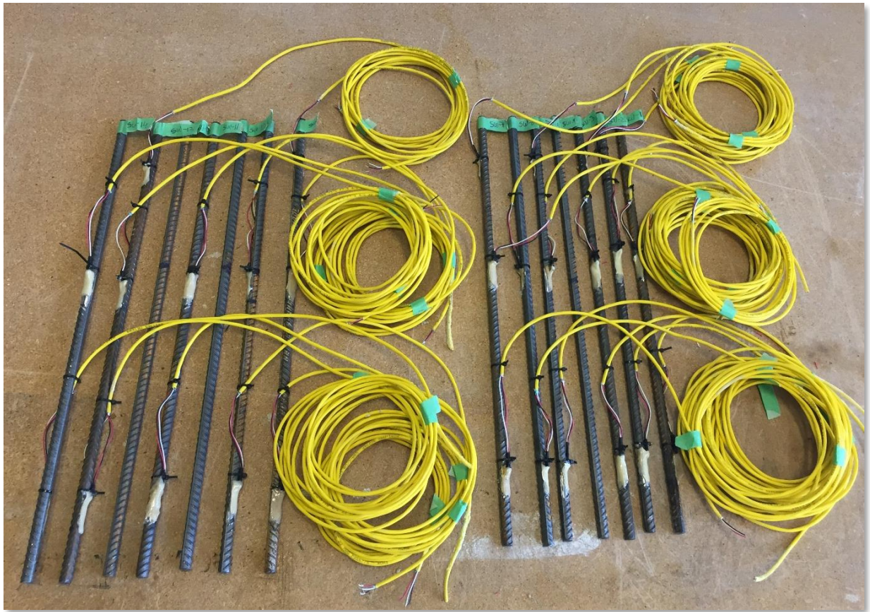
Figure 4.37 Installation of strain gauges on new segments of steel bars
