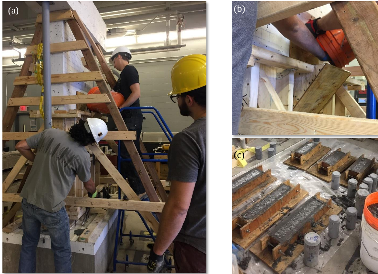
Figure 4.29 Procedure in Casting: (a) Casting of the wall; (b) pouring of ECC through the designed compartment; and (c) additional prisms and cylinders
