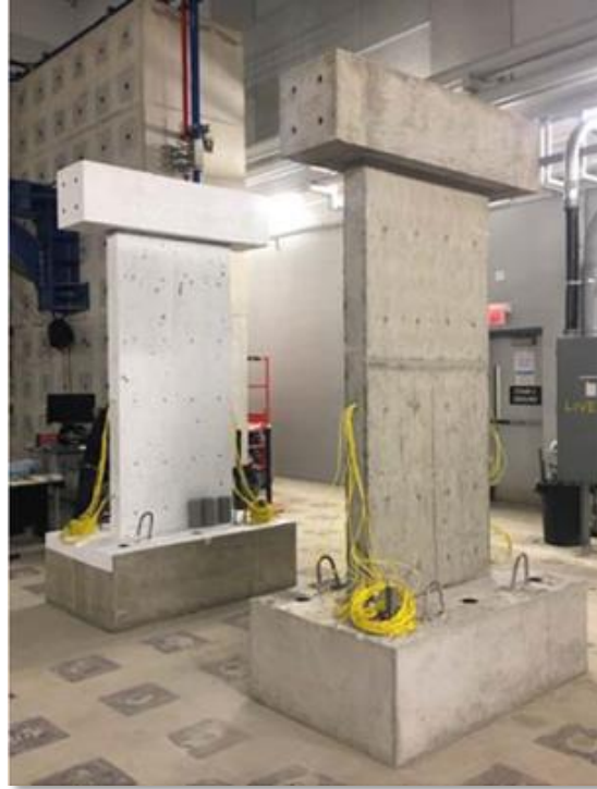
Figure 3.4. Walls after casting: SWS-R (behind) and SWN (forward) (Morcos and Palermo, 2018)
