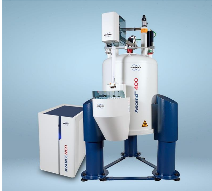
Figure 1-2 An actual NMR spectroscopy system [32]
