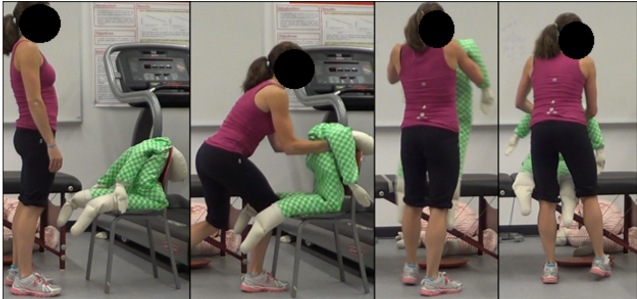
Figure 3.2. In the simulated patient transfer task, the participant moved the manikin from a seated position in the chair to a seated position on the massage table.
