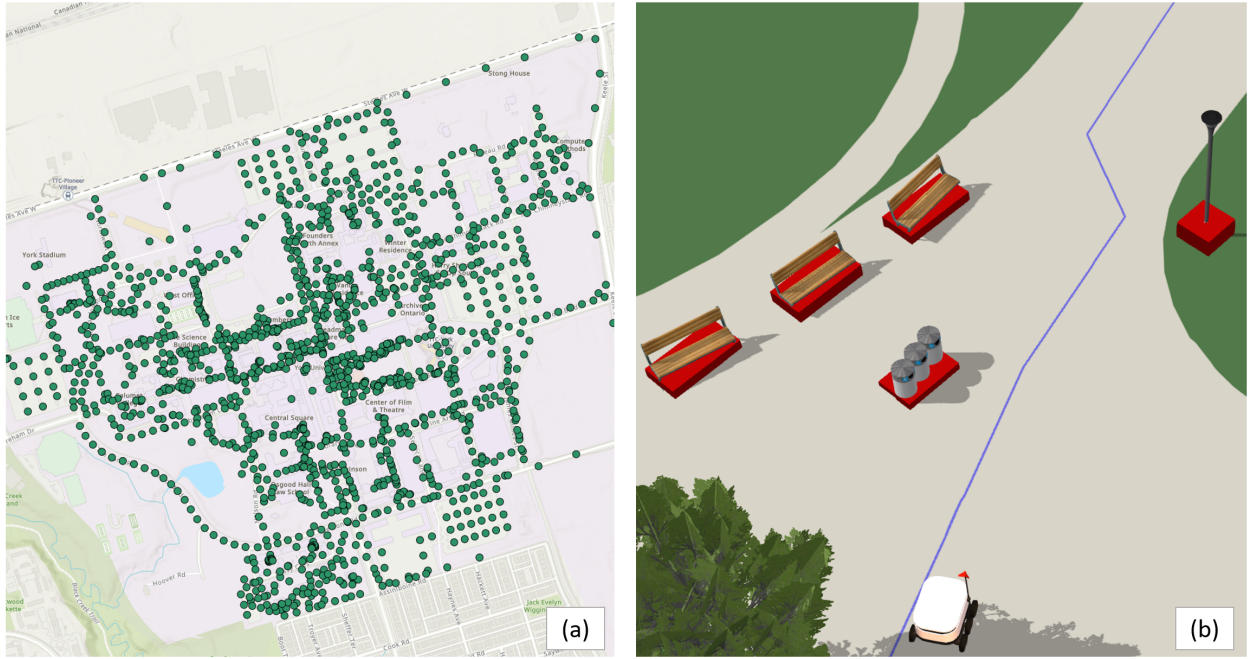
Figure 4.2: Visualization of Street Furniture Position Points: ArcGIS Hosted Layer Display- ing Critical Information Including Position, Dimensions, and Size (a), and Corresponding Bounding Boxes Created through Querying the Hosted Layer (b).
