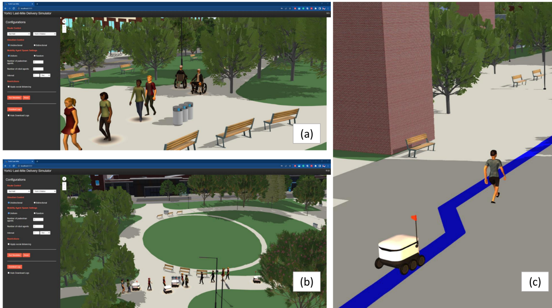
Figure 4.7: Last Mile Delivery Robot Simulation Tool: (a) and (b) show diverse mobility agents, including robots, pedestrians, and wheelchair users, seamlessly progressing to their destinations. In (c), agents adhere to the path created by the route analysis API.
