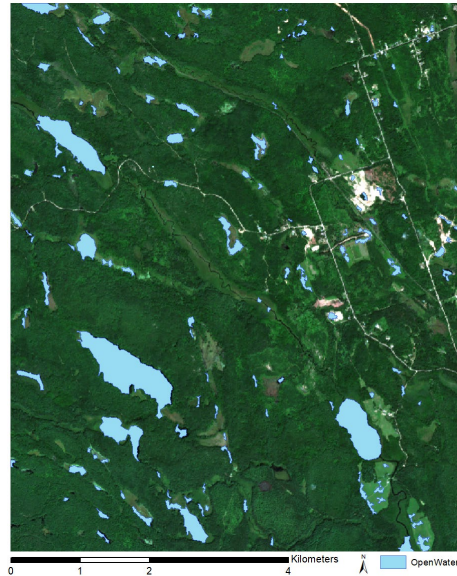
Figure 5.3. Open water bodies extracted from the seasonal RS2 data are shown in blue-lined polygons and overlaid on the S1 MSI summer scene, with the red band display in red, the green band display in green, and the blue band display in blue.
