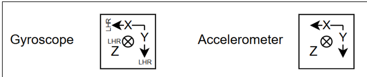
Figure 4-5: Frame of reference for the gyroscope and accelerometer of the IMUs. This frame is correct relative to the IMUs in the images shown in Figure 4-6 and Figure 4-8, i.e. for both IMUs, X acceleration is positive to the left and Y acceleration is positive to the bottom. We do not concern ourselves with the Z axis, as most of our obvious movements occur in the XY (sagittal) plane. For the gyroscope, counterclockwise rotation in the (XY) sagittal plane is positive, and clockwise rotation is negative. For more information on the reference frame of the DCU see EMBEDDED SYSTEM.
