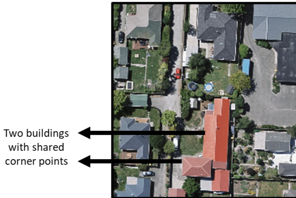
Figure 7.16 Adjacent Buildings with Shared Corners
