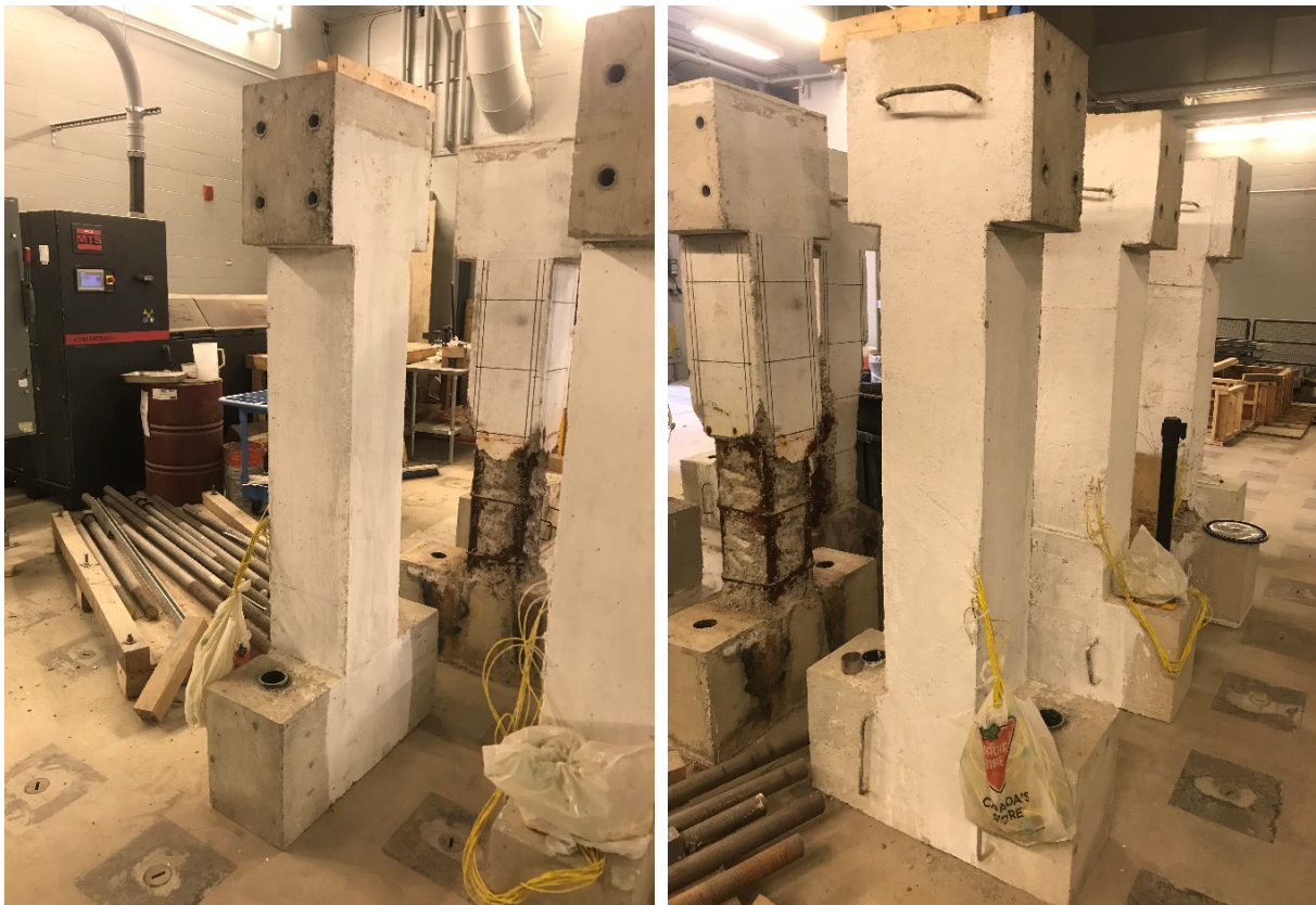
Figure C.11. Preparation of strengthened specimens for concrete removal.
