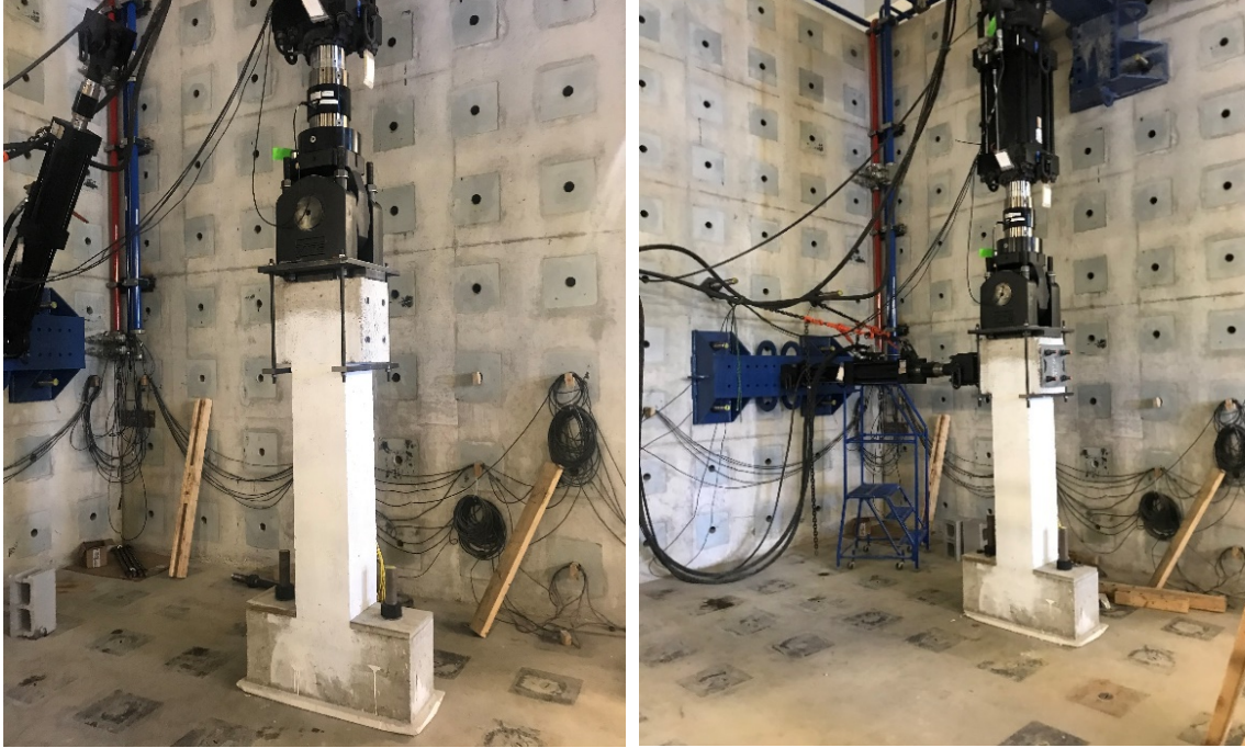
Figure 6.11. Setup of column specimens with only the axial actuator (left) and with both actuators (right). After fastening of the base, the columns were attached to the double actuator system, as shown in Fig. 6.11. The horizontal actuator was extended, using the MTS proprietary software for control, and the threaded steel rods were fastened through the two steel plates, on each side of the cap beam. For the axial actuator, the bottom head was lowered and fastened to the cap beam, using the threaded rods and plate connection shown in Fig. 6.11.
