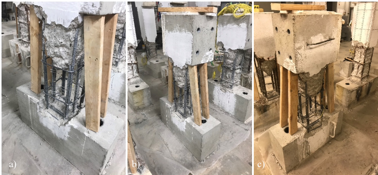
Figure C.5. Removal of damaged core from specimen CS3-15M-R: a-b) Front view; c) Back view.
