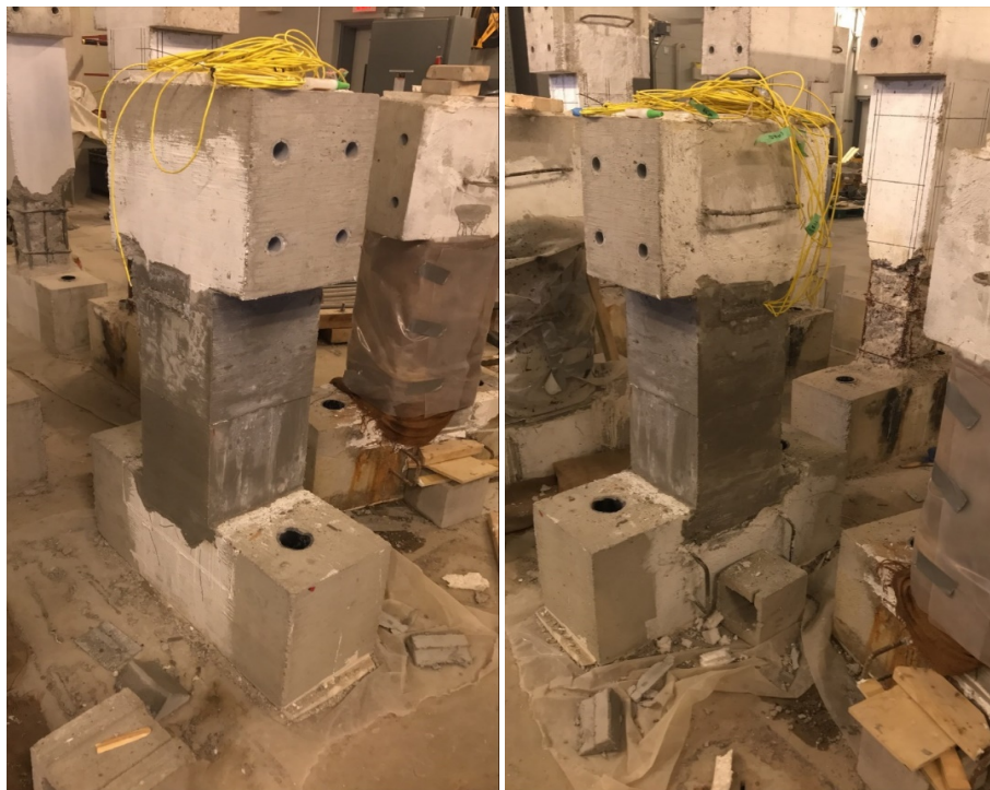
Figure 7.10. Retrofitted specimen with UHPFRC jacket, after removal of formwork, at two days.
