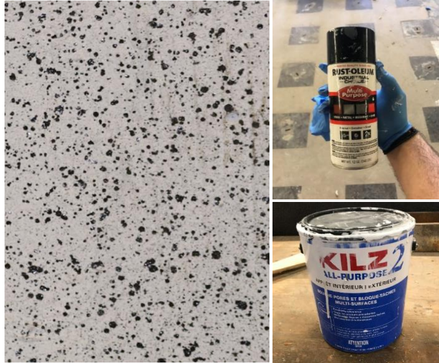
Figure 4.6. Left: Black-speckled surface for DIC analysis. Top-Right: Rust-Oleum black spray used for speckles. Bottom-Right: White Kilz primer used for jacket surface.
