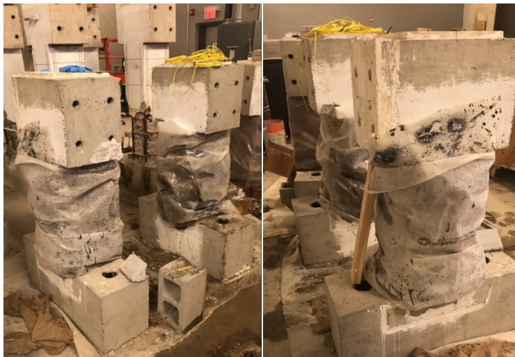
Figure 7.11. Covering of UHPFRC jacket with soaked burlap and plastic sheets for moisture retention.
