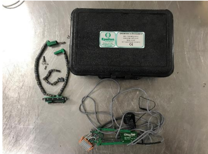
Figure 4.8. Epsilon chain-link circumferential extensometer for CC specimens.
