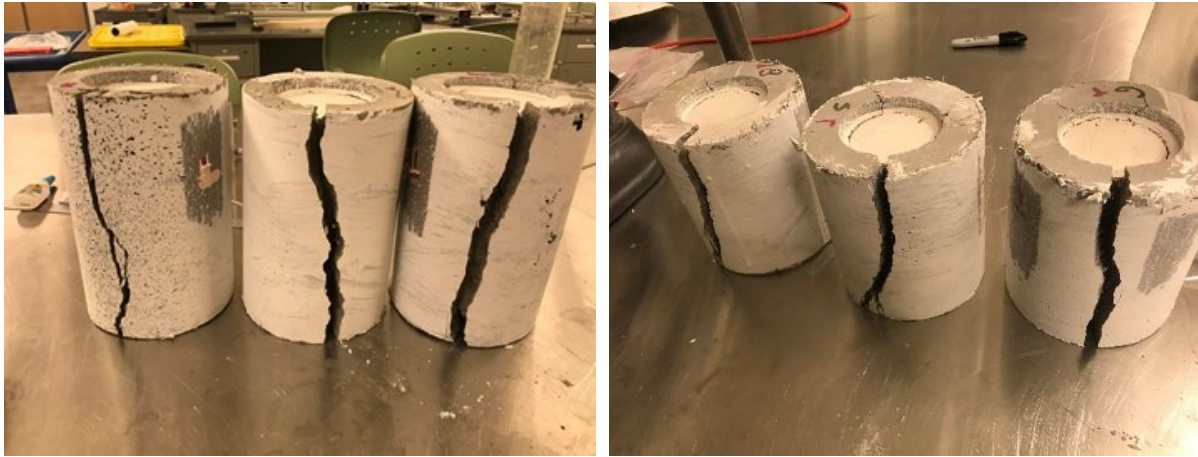
Figure 4.11. Distinctive vertical crack due to lateral expansion of the jacket; Left: CC25 specimens. Right: CC375 specimens.
