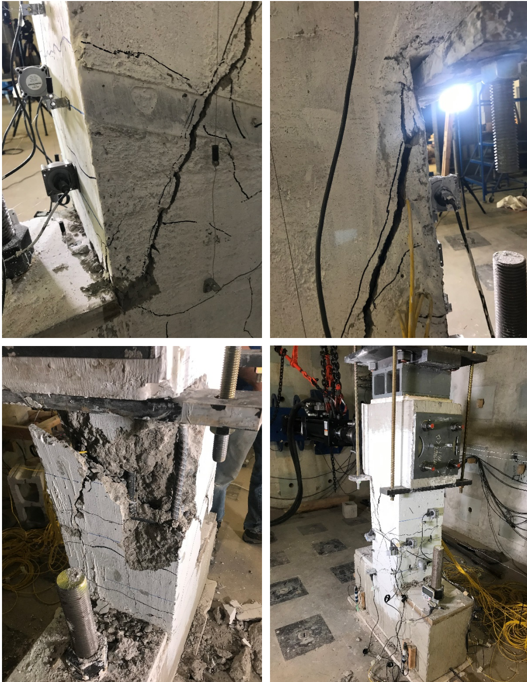
Figure C.16. Sides of specimen CS3-15M after termination of test.
