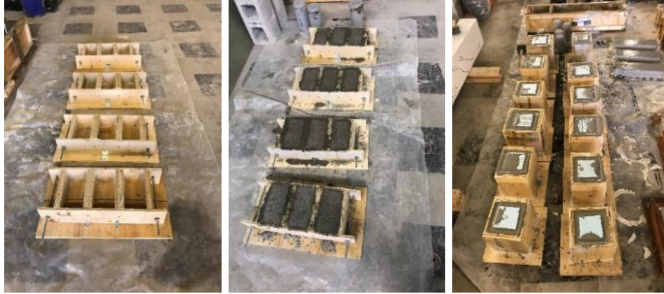
Figure 4.4. Specimen formworks for Confined Prisms: Casting of inner cores and UHPFRC jackets.
