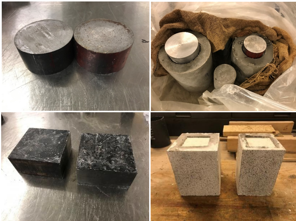
Figure 4.7. Left: Custom-fitted steel prisms for CC and CP specimens. Right: CC and CP specimens with plaster layer and speckled surface for DIC.
