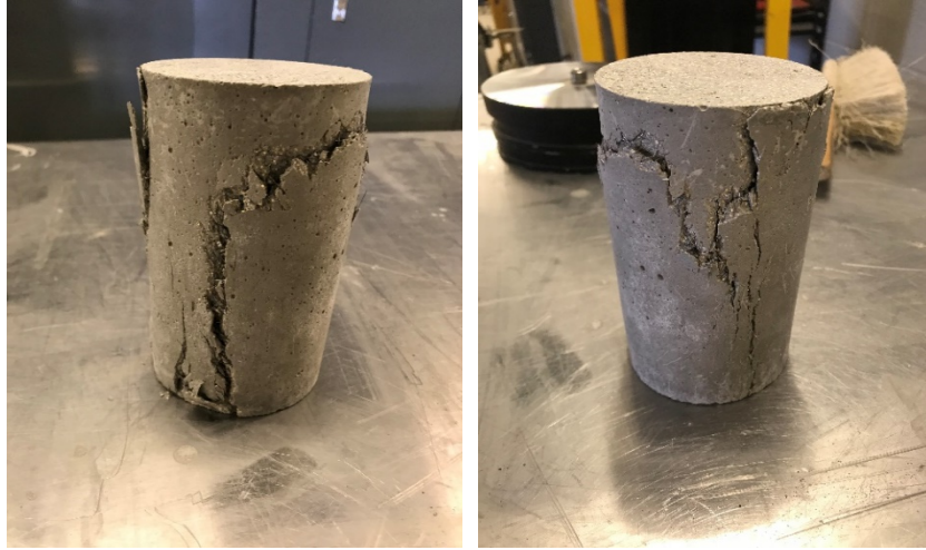
Figure 7.12. Cracked 75mm × 150mm UHPFRC cylinder after compression test.
