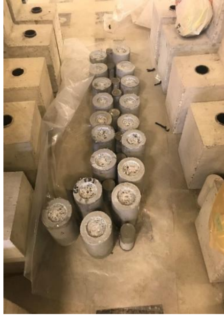
Figure 4.3. Confined cylinder specimens; Use of wet burlap for hydration; Custom steel cylinders for testing.
