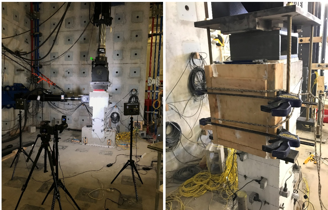
Figure 6.16. Complete modified setup for short column specimens (left); Attached formwork to improve leveling of side surface (right).
