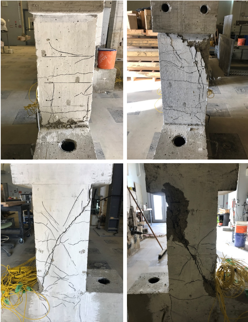
Figure C.17. Sides of specimen CS3-20M after termination of test.
