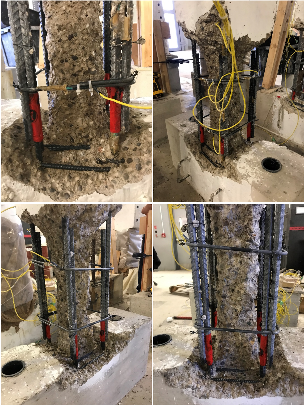
Figure C.13. Process of removal of cover and part of the core concrete for specimen CT1-20M-S.
