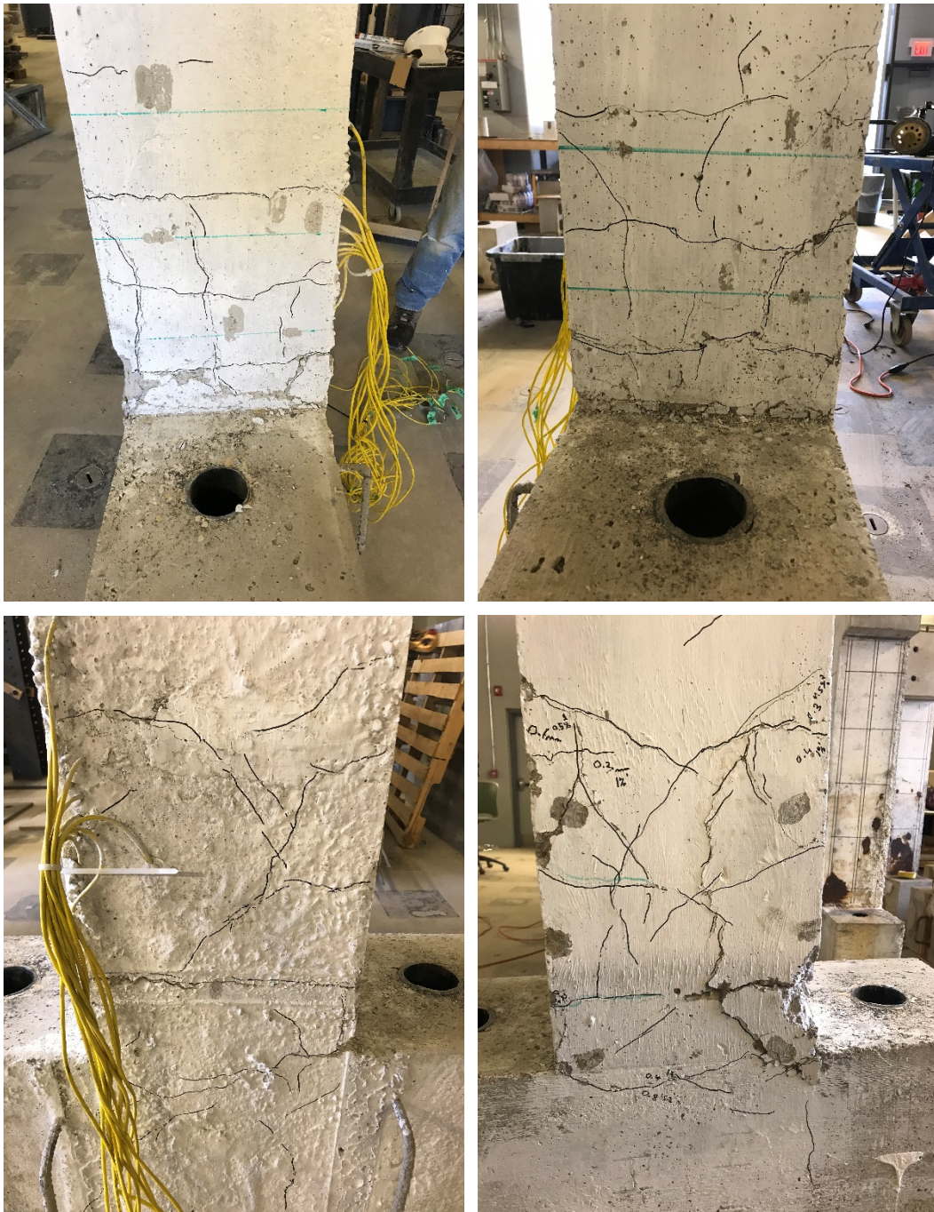
Figure C.14. Sides of specimen CT1-15M after termination of test.
