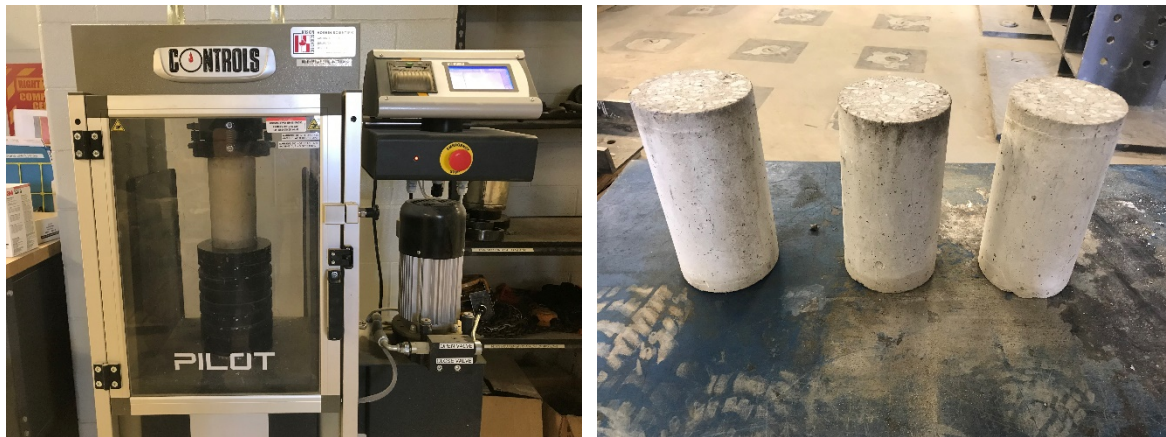
Figure 6.17. Compression testing of cylinders (left); Samples of cylinder specimens for testing (right).
