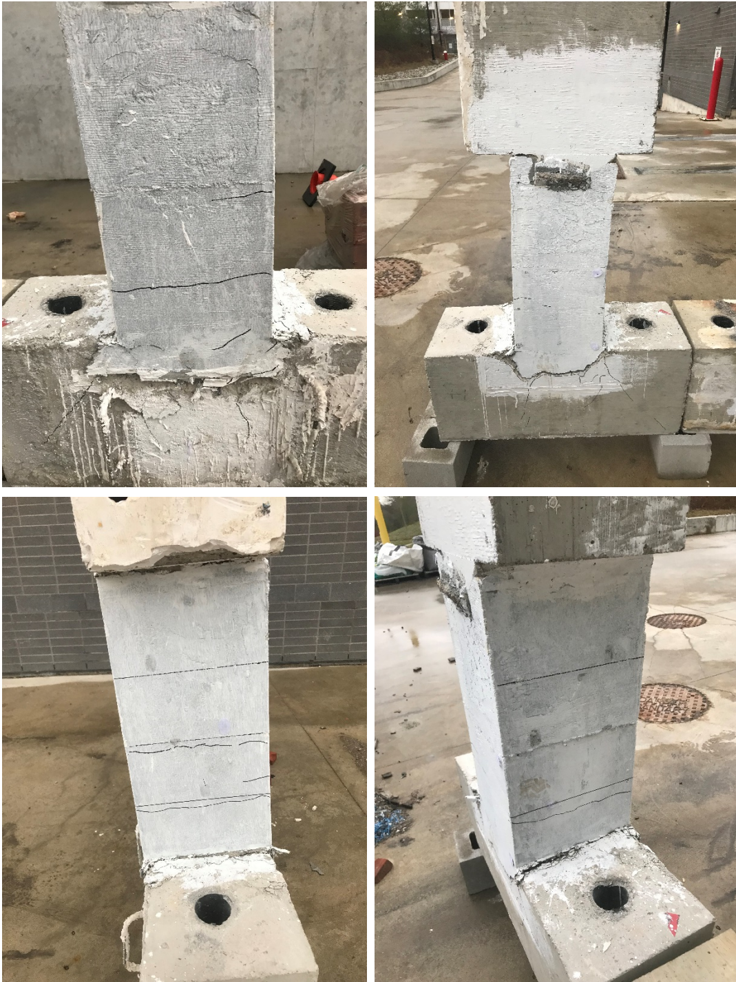
Figure C.23. Sides of specimen CS3-15M-R after termination of test.
