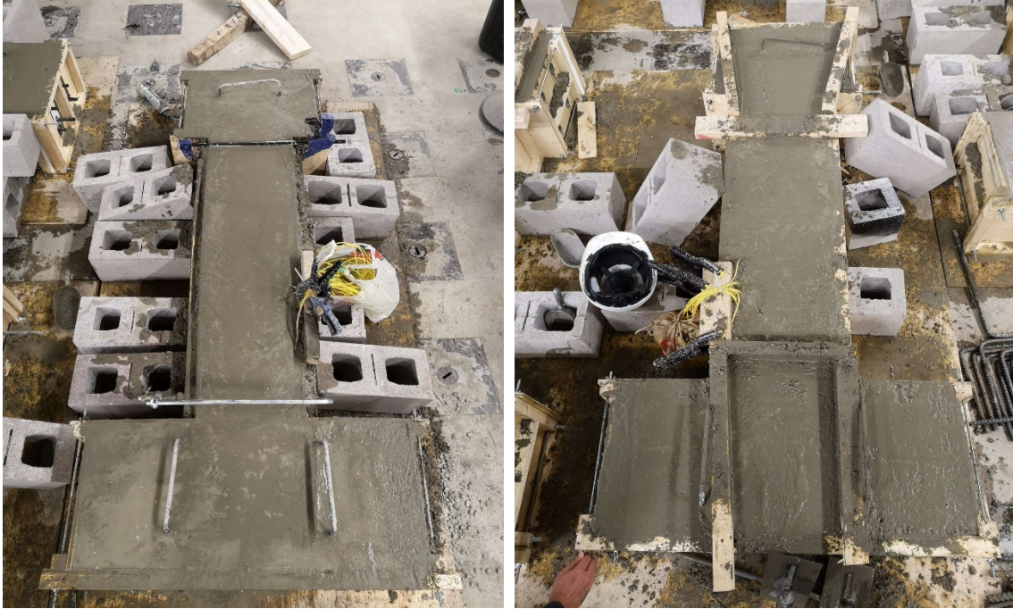
Figure C.2. Specimens after casting and prior to covering of the top surface.
