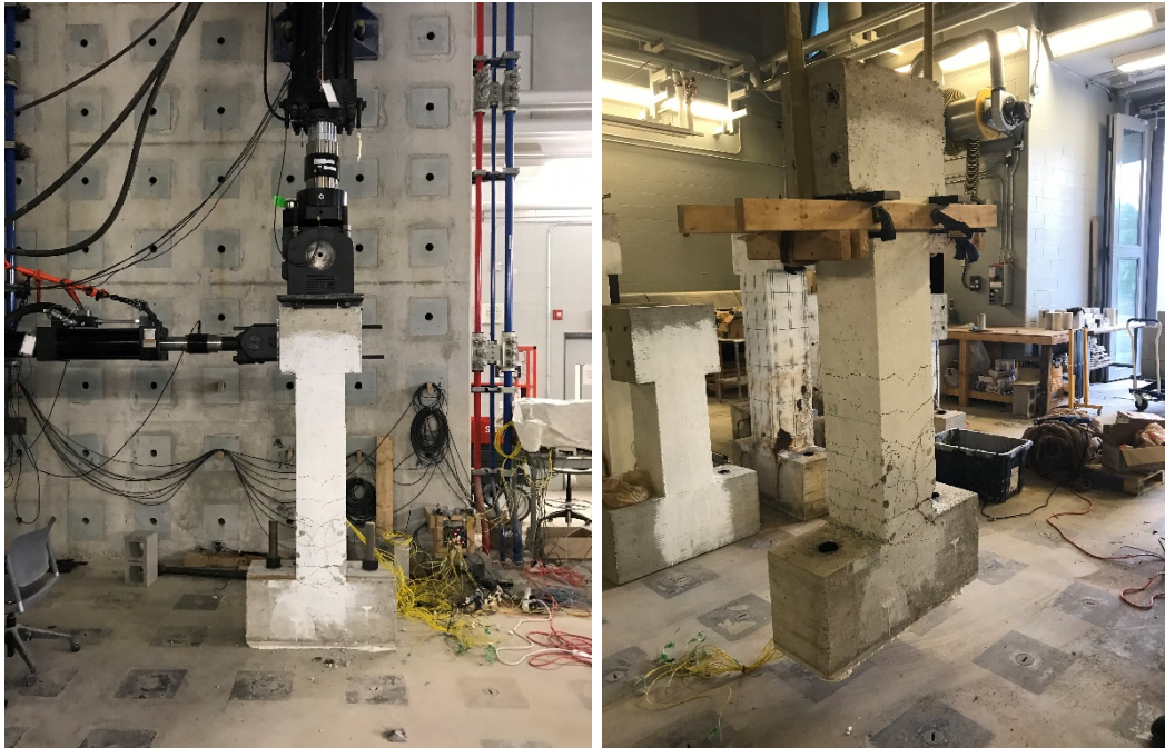
Figure 6.15. Column specimen after testing (left); Relocation of damaged columns to repair area (right).
