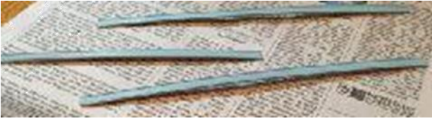
FIGURE 49. Warpage from painting one-side-only
