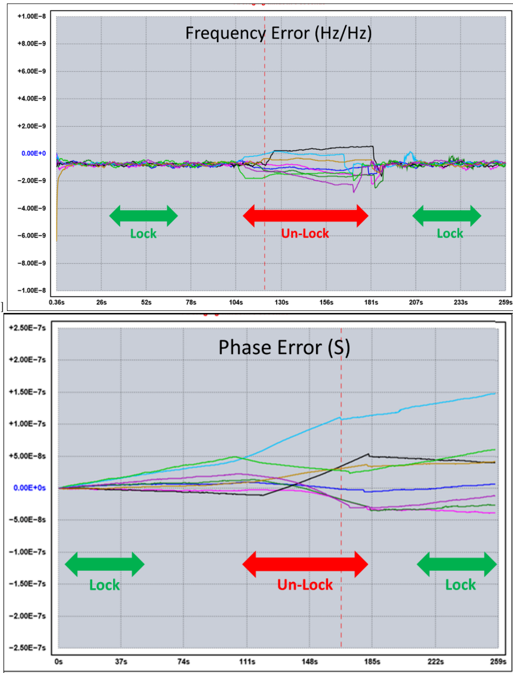
Figure 3.4: Example of frequency (top) and phase (bottom) errors after a loss of lock (Microsemi, 2018)
