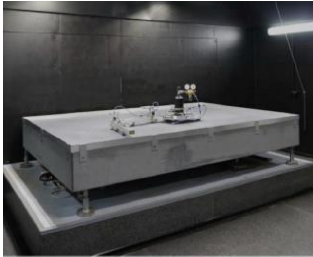
Figure 2.3 Planar air-bearing microgravity simulator [69].
