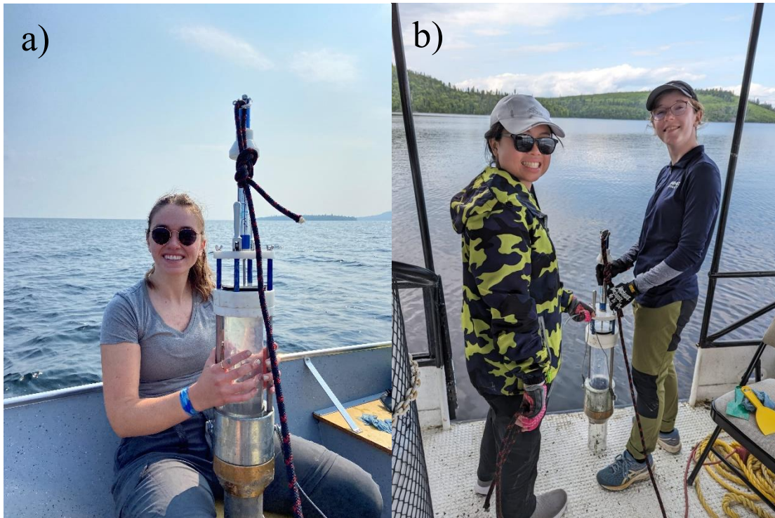
Figure 4.2. Sediment cores collected using a UWITEC™ gravity core on (a) a small fishing tugboat on Nipigon Centre and (b) the Velma Linda on Ombabika Bay.
