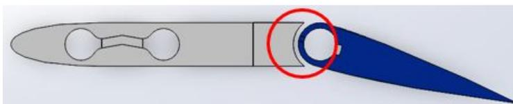
Figure A.4: Top view of the airfoil assembly with the gap (approx. 0.5 mm) circled in red.
