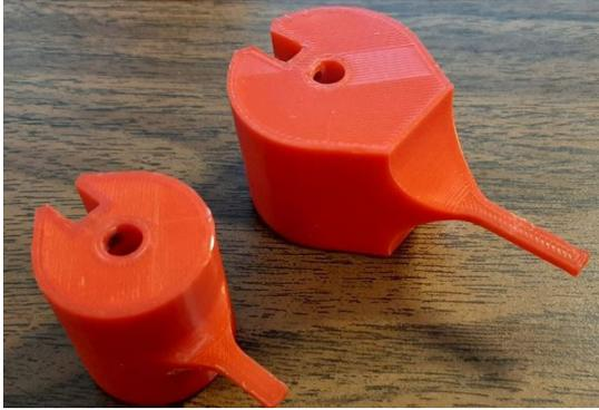
Figure 3.10: Equivalent MOI test mass (left) and the 4x MOI test mass (right).
