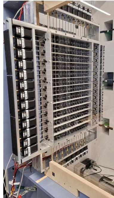
Figure 5.1: TGS installed onto the wind tunnel nozzle.
