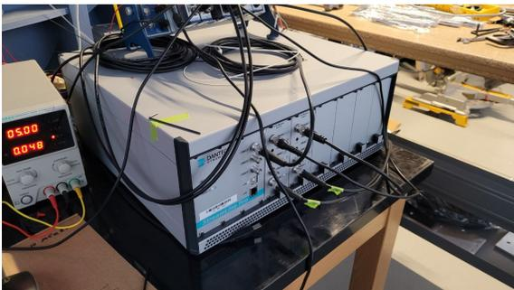
Figure 5.5: Dantec Streamline Pro used for setting up and conducting hotwire measurements.
