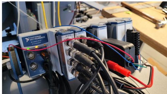
Figure 5.6: National Instruments data acquisition system used for data collection.
