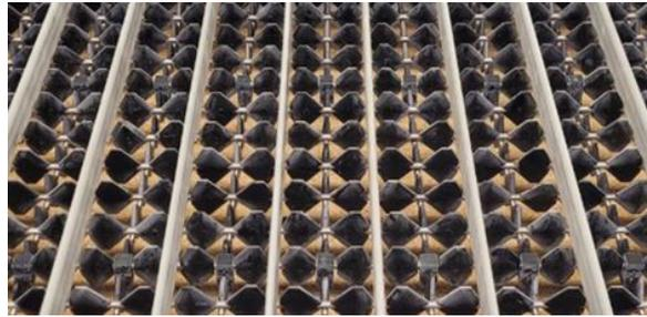
Figure A.2: Close up of the TGS in the fully open position. The fixed vertical active grid elements are shown to be in parallel to the airfoils. These elements remained fixed during the original tests.
