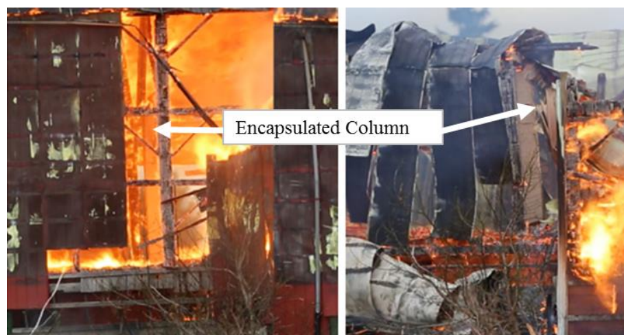
Figure 4.13 Images of Column 1 during field test (left) prior to structural collapse (right) post flashover event.
