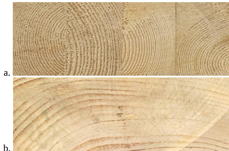
Figure 5.5 Cross sections of showing the growth ring width of, a. contemporary Glulam and b. historic timber, from a building constructed in the 1840s (author's photos).
