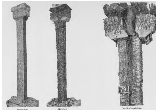
Figure 5.4 Qualitative results of the fire testing of one of the specimen, an unprotected longleaf pine column with a cap and pintle bearing (from [75]).
