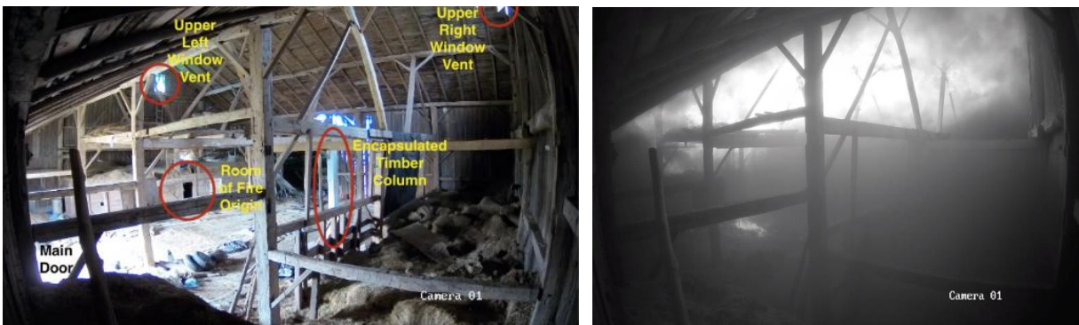
Figure 4.12 Pre heating view of compartment prior to fire ignition (left), atmosphere of compartment when fire spreads to column (right).
