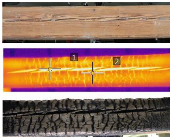
Figure C.7 Side A crack progression before (top) and after fire (middle and bottom) on Heritage 2 (identifiable markings were recorded temperature markers).
