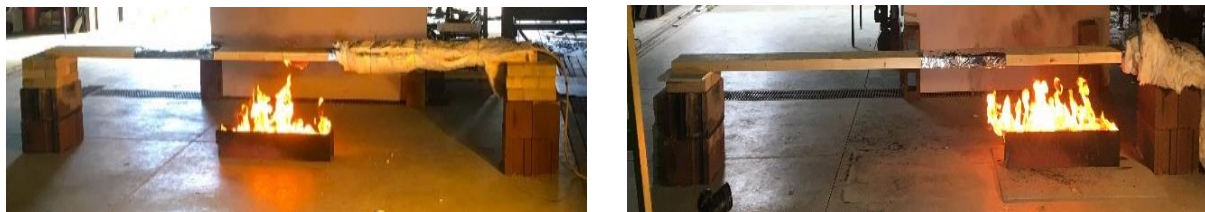
Figure 6.1. Test setup of the heating portion of the experiment for the moment region (left) and the shear region (right).
