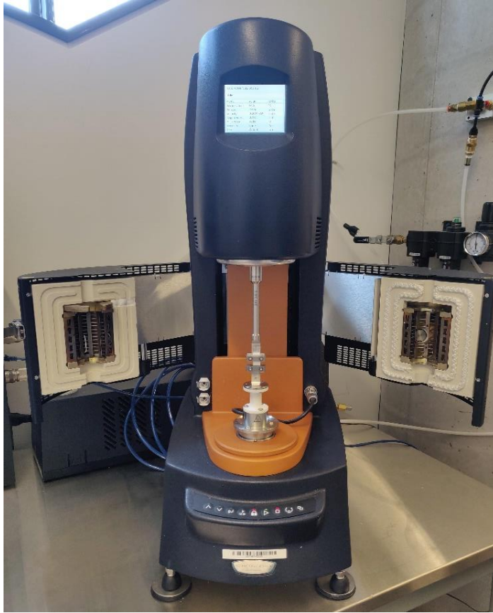
Figure 3.7 TA instruments Discovery Hybrid Rheometer (HR30) with tensile fixture installed.
