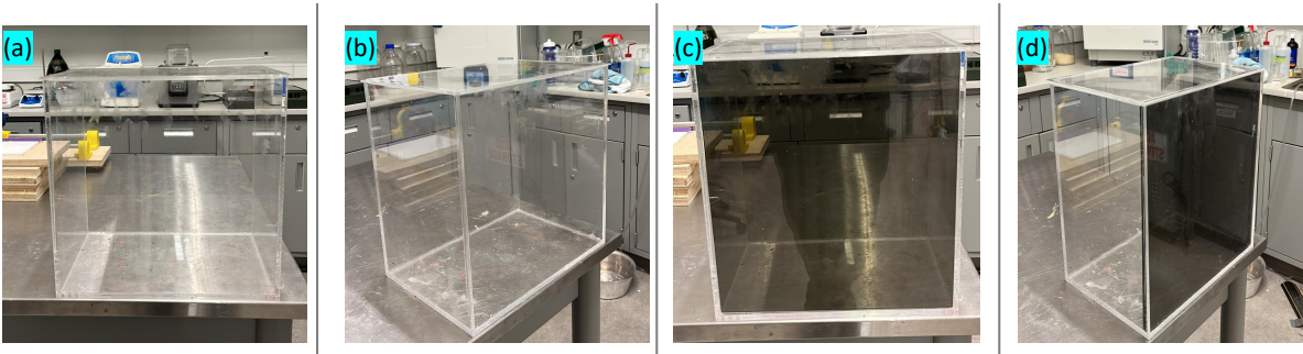
Figure 3.7 (a) Acrylic plexiglass water container (front view) (b) Acrylic plexiglass water container (view of side and front) (c) Acrylic plexiglass water container with tinted acrylic sheet (front view) (d) Acrylic plexiglass water container with tinted acrylic sheet (view of side and front)
