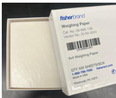
Figure 3: Cellulose-based weighing paper (Fisher brand, 4×4 inch) used as the substrate material for coated precursor films for laser carbonization and subsequent formation of laser-induced graphene (LIG).
