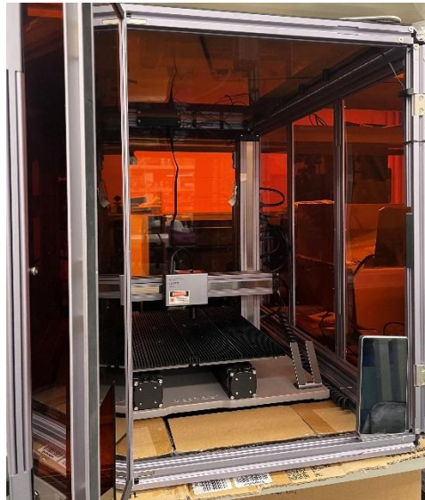
Figure 5: The Snapmaker 2.0, A350T 3in1 laser machine.
