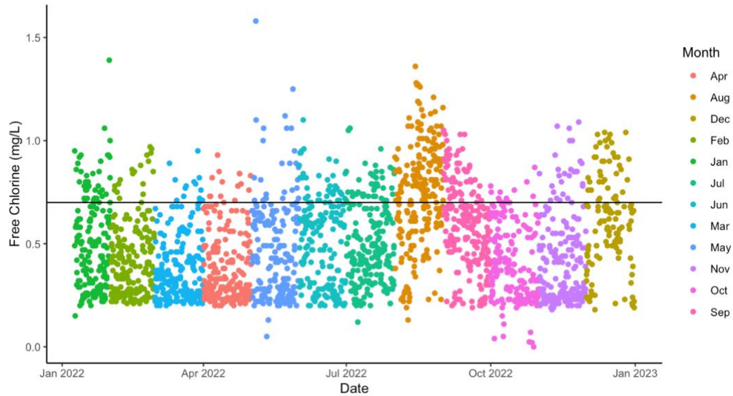
Figure F4-3: Continuous monitoring of free chlorine residual during 2022, provided by GN-CGS WaterTrax management system. The black line represents the recommended free chlorine residual level of 0.7 mg/L
