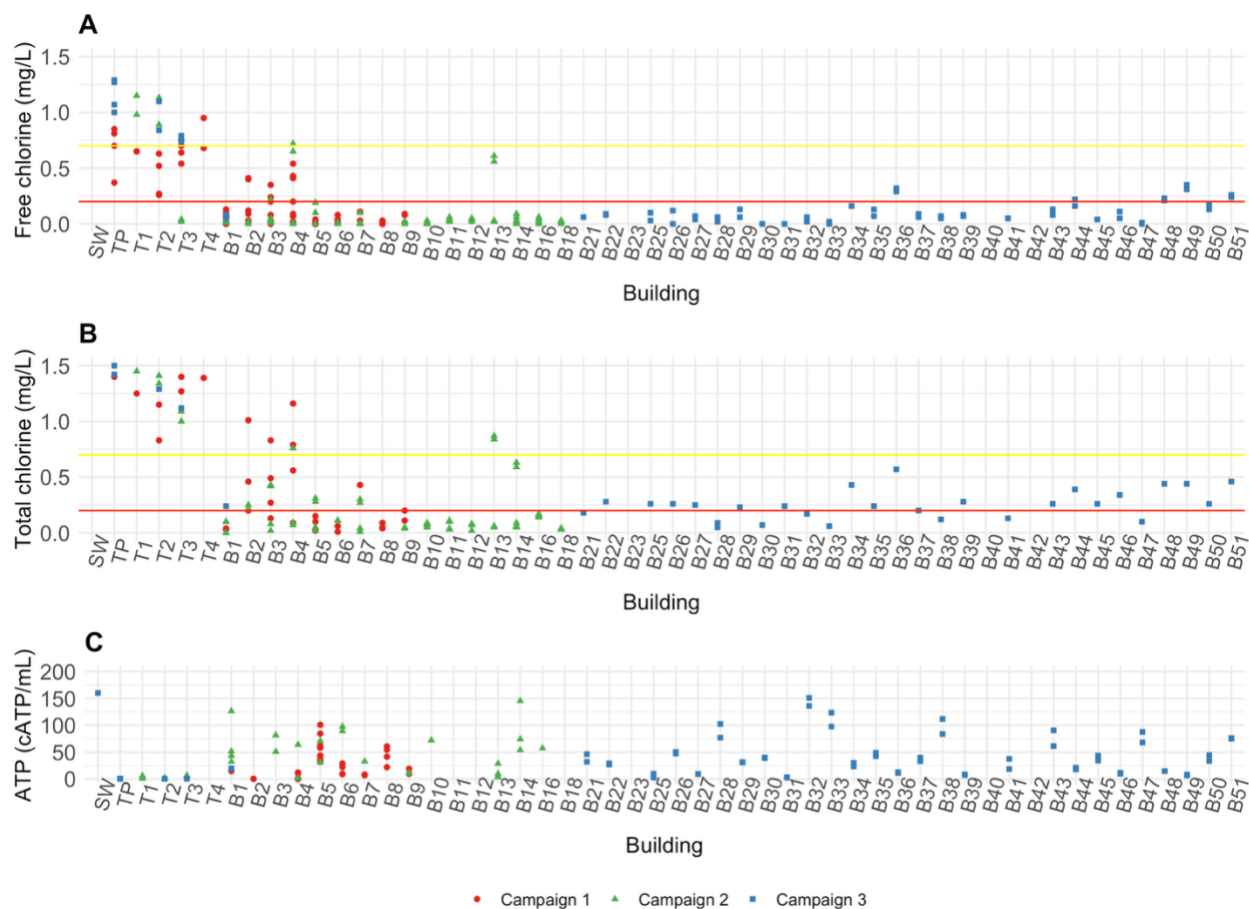
Figure 5-2: (A) Free chlorine, (B) total chlorine, and (C) ATP measured in water samples collected from various locations in the water system in Cambridge Bay, NU during different seasons. The red line shows the current Government of Nunavut regulatory requirement of 0.2 mg/L of free chlorine and the yellow line is the recommended free chlorine residual at 0.7 mg/L leaving the WTP to achieve log-4 removal of viruses through disinfection. Acronyms: SW- Source Water, TP – Treatment Plant, T1-4 – Trucks, B – Building.
