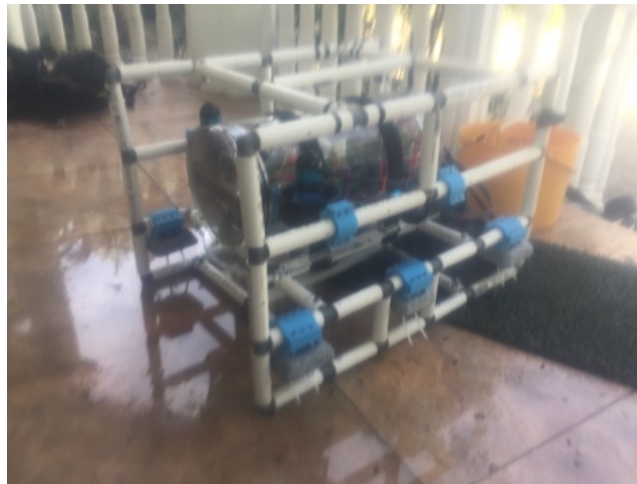
Figure 3.4: Milton shows the Milton robot fully assembled on the bench. The mounting points for the ballast weights and the 3d printed mounting points for the thrusters are shown.
