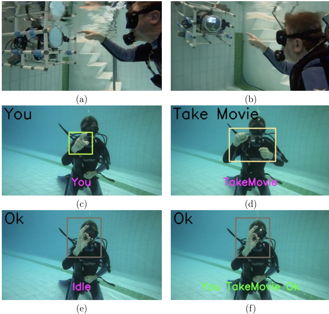
Figure 1.6: Gesture Detection and Feedback
