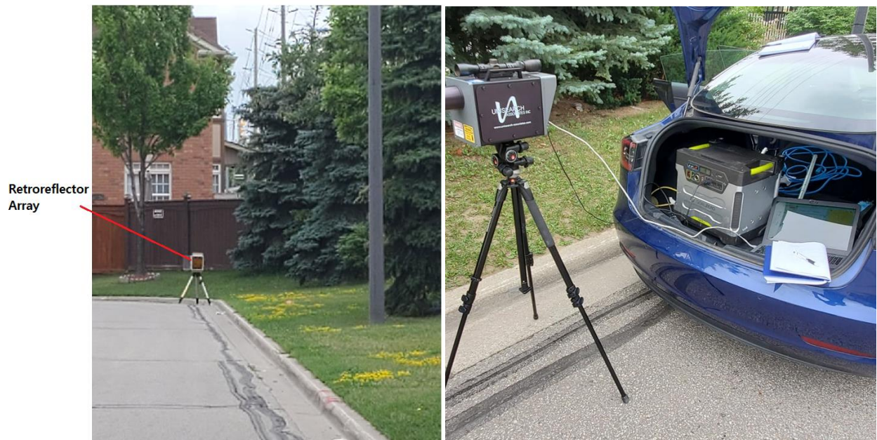
Figure 2.7: Pictures showing the set up of TDL at measurement downwind location 1 where retroreflector was placed 56 m away from the TDL instrument powered by the battery mounted in a car.
