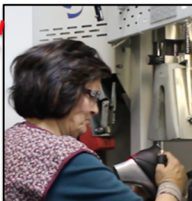
Figure 35 Production: First Trial - counter molding the heel with Katarina and Nelson Silva, photographed at Mellow Walk, December 20, 2013.
