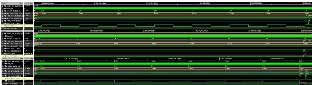
Figure 2.12: Post-Synthesis Simulation of the gcd_encoder block
