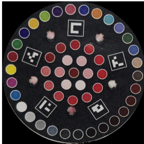
Figure 3.2: The calibration layer fitted onto the sweat patch, illustrating the swatches, chamber cutouts, and ArUco markers as physical features.
