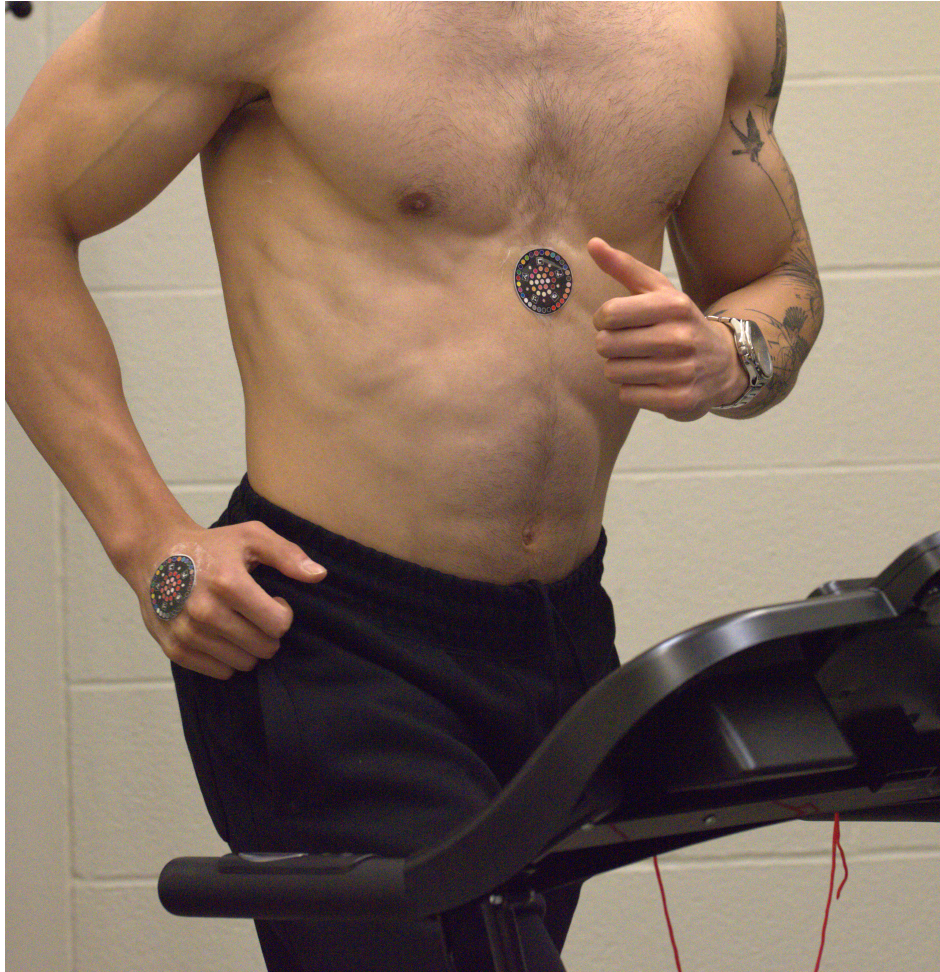
Figure 3.16: On-body clinical evaluation of the device in healthy and patient cohorts with sweat-collection protocol during brisk walking on a treadmill (4 miles per hour (mph)).
