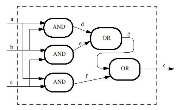
The circuit is intended to implement a vote(a, b, c) function which returns true if the two or more of the inputs a, b, c are true. We want to verify this by showing that if the inputs are translated to integers 1 or 0 and summed, the sum of the inputs (as integers) is 2 iff z is true.
